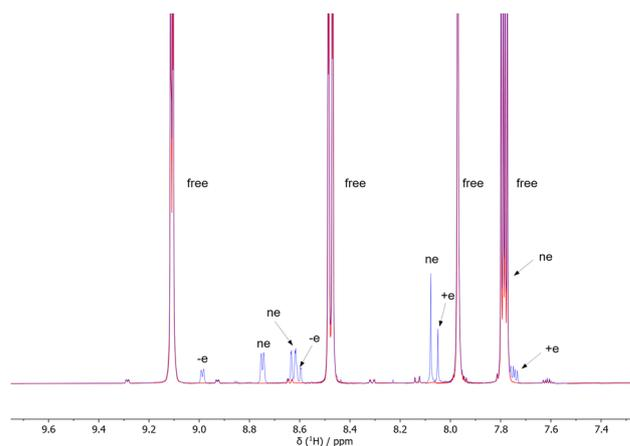
Fig. 3 500 MHz  $^1\text{H}$  NMR subspectrum of 10 mM 1,10-phenanthroline and 1 mM  $[\text{IrCl}(\text{COD})(\text{IMes})]$  in  $\text{CD}_3\text{OD}$  before (red) and after (blue)  $\text{H}_2$  pressurization (3 bar). The letters indicate the signals of phenanthroline bound to the Ir complex that provide positively enhanced (+e), negatively enhanced (−e) or non-enhanced (ne) signals under SABRE conditions. The label free indicates free phenanthroline in solution.
