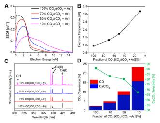
Fig. 5 (A) Simulated electron energy distribution functions and (B) simulated average electron temperatures under varying CO<sub>2</sub>/Ar compositions. (C) Optical emission spectra (300-450 nm) of Ca and •OH spectral lines and (D) CO<sub>2</sub> conversion and CaCO<sub>3</sub> selectivity as a function of CO<sub>2</sub> mole
