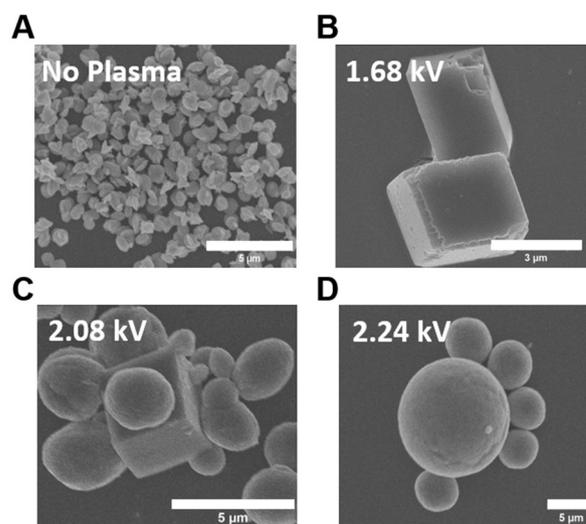
Fig. 3 Scanning electron micrographs of precipitated  $\text{CaCO}_3$  at different discharge voltages showing the influence of phase purity on  $\text{CaCO}_3$  morphology. (A) Ellipsoidal vaterite, (B) rhombohedral calcite, (C) spheroidal and rhombohedral vaterite and (D) spherical vaterite.
