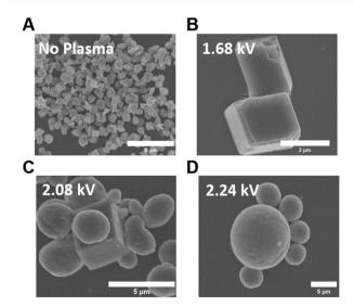
Fig. 3 Scanning electron micrographs of precipitated  $CaCO_3$  at different discharge voltages showing the influence of phase purity on CaCO<sub>3</sub> morphology. (A) Ellipsoidal vaterite, (B) rhombohedral calcite, (C) spheroidal and rhombohedral vaterite and (D) spherical vaterite.
