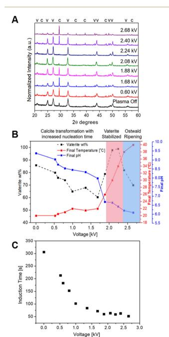
Fig. 2 (A) Powder X-ray diffraction of precipitated CaCO<sub>3</sub> at different plasma discharge voltages. (B) Discharge voltage-dependent formation of vaterite (wt%) and the final temperature and pH of the bulk solution after 5 minutes of plasma exposure. (C) Induction time at various applied plasma voltages. The induction times observed occur at pH values ranging from 10.00 to 9.50
