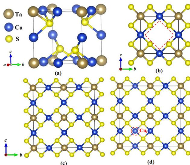
Fig. 1 Unit cell of  $\text{Cu}_3\text{TaS}_4$  (a). The unit cell of  $\text{Cu}_3\text{TaS}_4$  viewed from the (100) direction (b). The  $2 \times 2 \times 2$  supercell of  $\text{Cu}_3\text{TaS}_4$  (c). The  $2 \times 2 \times 2$  supercell of  $\text{Cu}_3\text{TaS}_4$  with a  $\text{Cu}_i$  (marked by a red dotted circle) in the empty “channel” (d).
