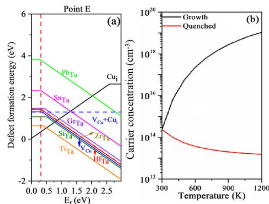
Fig. 6 The defect formation energies (a) of p-type doping at the Ta site as a function of the Fermi level at point E. The red vertical dotted line represents the Fermi level at 300 K with  $\text{Ti}_{\text{Ta}}$ . The hole concentration as a function of growth temperature with  $\text{Ti}_{\text{Ta}}$  at point E (b).
