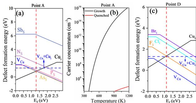
Fig. 7 The defect formation energies (a) of p-type doping at the S site at point A as a function of the Fermi level. The hole concentration with  $As_S$  as a function of growth temperature at point A (b). The defect formation energies of interstitial defects at point D as a function of the Fermi level (c). The red vertical dotted lines are the Fermi level at 300 K.
