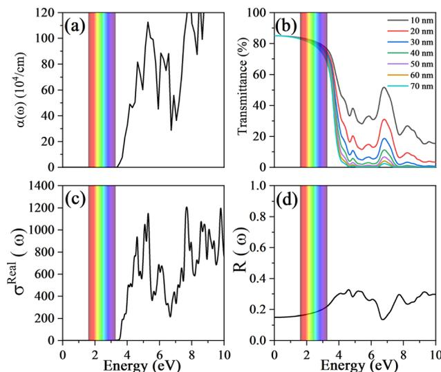
Fig. 3 The absorption coefficient (a), the optical transmittance as a function of film thickness (b), the optical conductivity (c) and the reflectivity (d) of Cu<sub>3</sub>TaS<sub>4</sub>.
