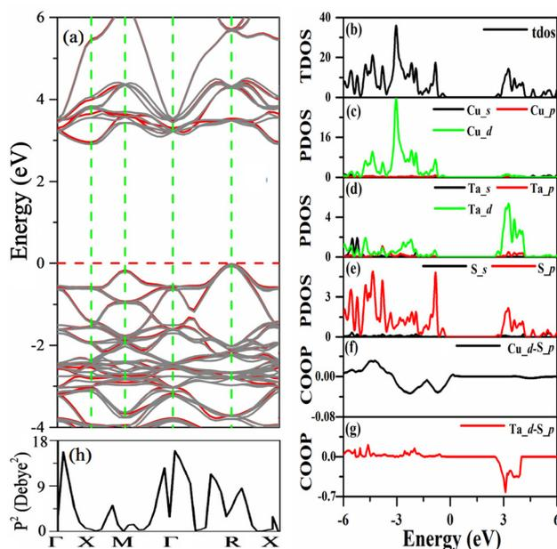
Fig. 2 The band structure of  $\text{Cu}_3\text{TaS}_4$  with (grey line) and without (red line) the SOC effect (a). The VBM is set to zero. The total density of states (b) and partial density of states of Cu (c), Ta (d) and S (e) atoms and COOPs between the Cu-d and S-p states (f) and the Ta-d and S-p states (g), respectively. The squares of the dipole transition matrix elements between the highest valence band and the lowest conduction band at various  $k$  points (h).
