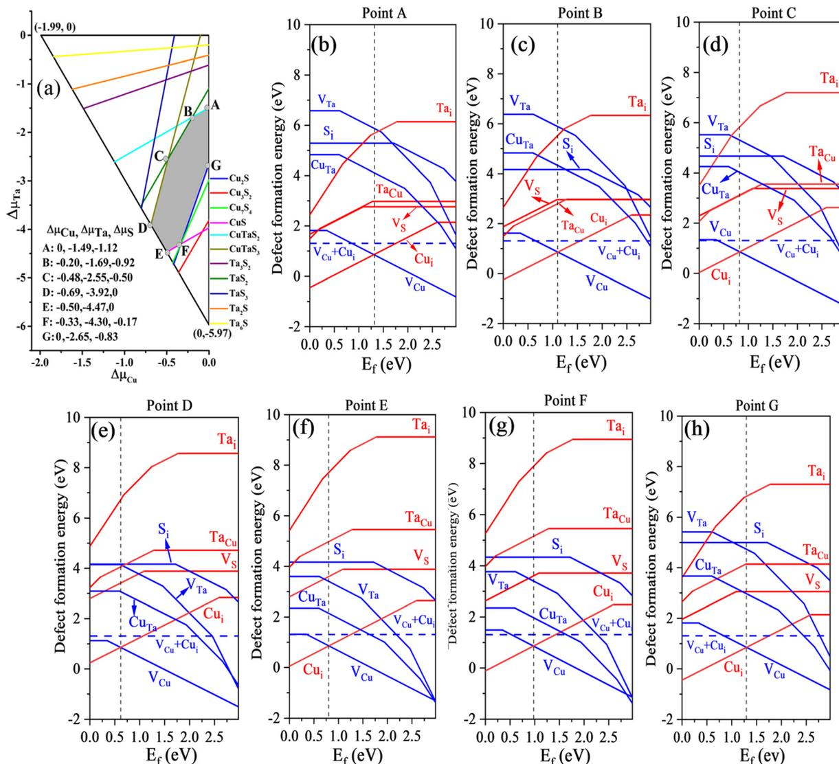
Fig. 4 The allowed range of relative chemical potentials for stable  $\text{Cu}_3\text{TaS}_4$  (a). The defect formation energies of  $\text{Cu}_3\text{TaS}_4$  as a function of the Fermi level under seven extreme chemical potential environments [(point A to point G) (b)–(h)]. The black vertical dotted lines represent the Fermi level at 300 K.
