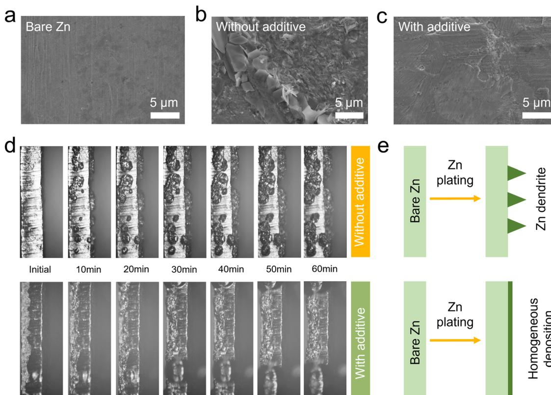
Fig. 2 SEM images of (a) bare Zn. SEM images of the Zn electrodes of Zn||Cu cells in (b) ZS and (c) AS electrolyte after 10 cycles under a current density of  $5.0 \text{ mA cm}^{-2}$  for 0.2 h. (d) *In situ* optical microscope observation of the Zn deposition process in ZS and AS electrolyte at the current density of  $5 \text{ mA cm}^{-2}$ . The right side and cross-section were observation surfaces. (e) A graph of Zn deposition in ZS/AS electrolyte.
