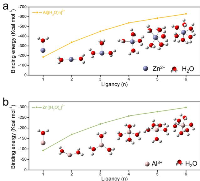
Fig. 6 DFT calculation studies of ion solvation binding energy in the electrolyte. (a) The binding energy as a function of representative Zn<sup>2+</sup> ion cluster models. (b) The binding energy as a function of representative Al<sup>3+</sup> ion cluster models.
