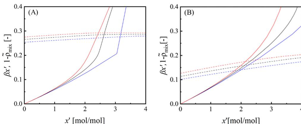
Fig. 9 Contribution of  $1 - \bar{p}_{\text{mix}}$  (dashed lines) and  $\beta x'$  (solid lines). (A) [emim][Tf<sub>2</sub>N] + CO<sub>2</sub> mixture (lines: blue, 298.15 K; black, 323.15 K; red, 343.15 K). (B): [emim][FAP] + CO<sub>2</sub> mixture (lines: blue, 303.15 K; black, 323.15 K; and red, 343.15 K).
