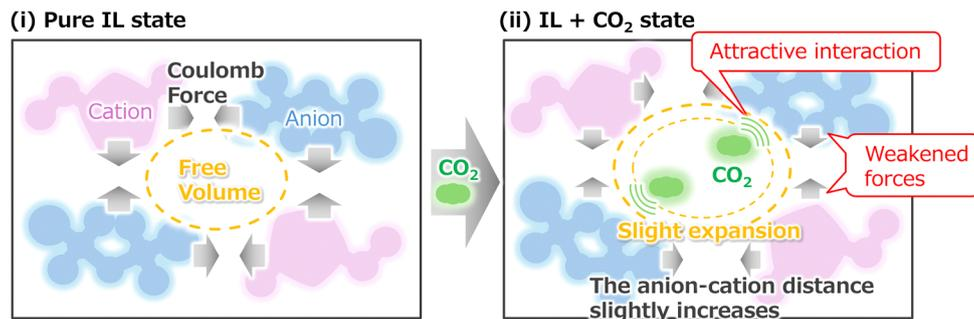
Fig. 8 The mechanism of viscosity reduction caused by CO<sub>2</sub> dissolution.
