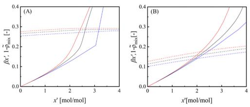
Fig. 9 Contribution of  $1 - \tilde{\rho}_{\text{mix}}$  (dashed lines) and  $\beta x'$  (solid lines). (A) [emim][Tf<sub>2</sub>N] + CO<sub>2</sub> mixture (lines: blue, 298.15 K; black, 323.15 K; red, 343.15 K). (B): [emim][FAP] + CO<sub>2</sub> mixture (lines: blue, 303.15 K; black, 323.15 K; and red, 343.15 K).
