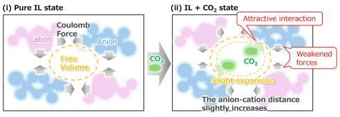
The mechanism of viscosity reduction caused by CO<sub>2</sub> dissolution.
