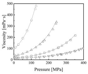
Fig. 3 Correlation results for viscosity of lemim1/Tf<sub>2</sub>N1.<sup>65</sup> Symbols: O. 273.15 K; Δ, 298.15 K;  $\square$ , 323.15 K;  $\nabla$ , 348.15 K. Lines: FVT + ε\*-mod SL-
