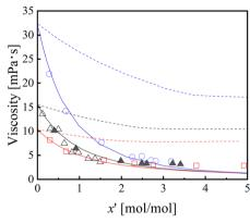
Fig. 6 Prediction and correlation results for the viscosity of the [emim][Tf<sub>2</sub>N] + CO<sub>2</sub> mixture. Symbols:  $\bigcirc$ , 298.15 K;<sup>43</sup>  $\triangle$ , 323.15 K;<sup>43</sup>  $\square$ , 343.15 K;  $^{43}$   $\blacktriangle$ , 323.15 K.  $^{44}$  Dashed lines: prediction with FVT +  $\varepsilon$ \*-mod SL-EoS ( $\beta$  = 0). Solid lines: correlation with FVT +  $\varepsilon$ \*-mod SL-EoS ( $\beta \neq 0$ ).
