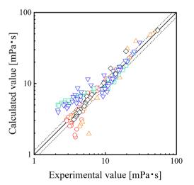
Fig. 7 Parity plot for the viscosity of the IL + CO<sub>2</sub> mixture. Symbols: O, [hmim][FAP] + CO<sub>2</sub> mixture. 44 Dashed lines: overall ARDs (14.3%; see Table 5) of the FVT +  $\varepsilon$ \*-mod SL-EoS model.
