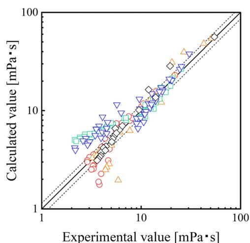
Fig. 7 Parity plot for the viscosity of the IL + CO<sub>2</sub> mixture. Symbols: ○, [emim][Tf<sub>2</sub>N] + CO<sub>2</sub> mixture;<sup>43</sup> △, [hmim][Tf<sub>2</sub>N] + CO<sub>2</sub> mixture;<sup>43</sup> ◇, [dmim][Tf<sub>2</sub>N] + CO<sub>2</sub> mixture;<sup>43</sup> ▽, [emim][FAP] + CO<sub>2</sub> mixture;<sup>44</sup> ▽, [hmim][FAP] + CO<sub>2</sub> mixture.<sup>44</sup> Dashed lines: overall ARDs (14.3%; see Table 5) of the FVT +  $\epsilon^*$ -mod SL-EoS model.
