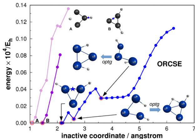
Fig. 10 ORCSE paths for  $C_3H_2$  and  $Si_3H_2$  searching for possible structural isomers as obtained by varying the distance between atoms separated by a star. With this bond treated as inactive coordinate, all other DOF are optimized, and energies measured relative to starting-geometry one. In this plot and that of Fig. 13, n.c. stands for non-converged.
