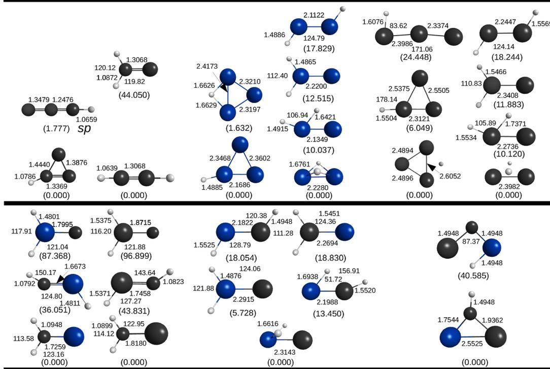
Fig. 7 Tetraatomic mono- and dihydrides of C, Si and Ge optimized at the CCSD(T)/AVTZ level of theory. Given in brackets are relative energies in kcal mol<sup>-1</sup>. Due to lack of space, not all relevant coordinates may have been indicated. They may be obtained from the ESI.† Also there are the harmonic vibrational frequencies.
