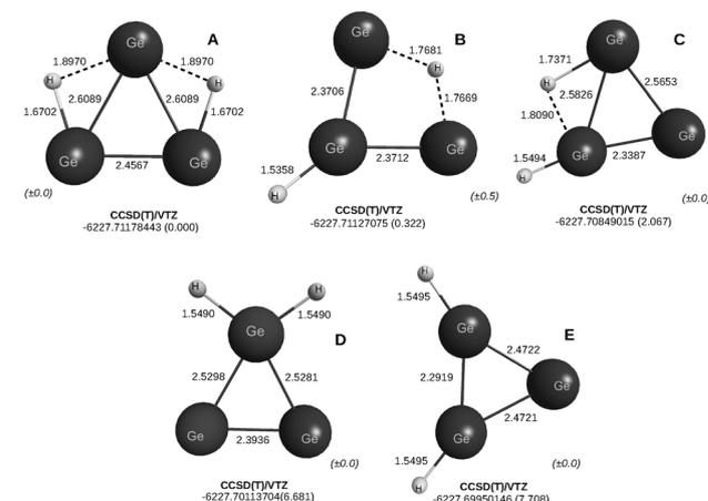
Fig. 12 CCSD(T)/AVTZ geometries and energies of five lowest isomers ( $\leq 20$  kcal mol $^{-1}$ ) of  $Ge_3H_2$ . Indicated at the bottom right-hand-side corner of each structure is the maximum deviation found in the two dihedral angles.
