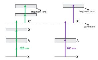
Fig. 2 Fenchone energy level diagram and ionization schemes for the 520 nm and 260 nm laser pulses. X and X' are the ground states of the fenchone neutral and cation, A is the  $\pi^*$  first excited state of the neutral, with the D band also shown. The generation of fragments by absorption of 2  $\times$  520 nm photons or 1  $\times$  260 nm photon is only indicative and is more likely to proceed if further photons are absorbed.
