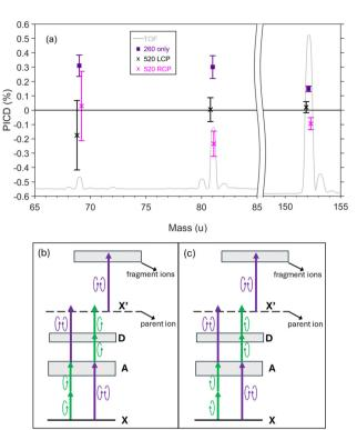
Fig. 9 (a) Two-colour PICD of (+) fenchone derived from the differences in ion yields from changing the 260 nm polarization between LCP and RCP while the polarization of the 520 nm is fixed at: LCP - black cross; RCP magneta cross. Plotted for comparison are the one-colour 260 nm only PICD values – purple squares. (b) and (c) the two-colour ionization pathways where for each measurement the 520 nm polarization was fixed at LCP and RCP respectively.
