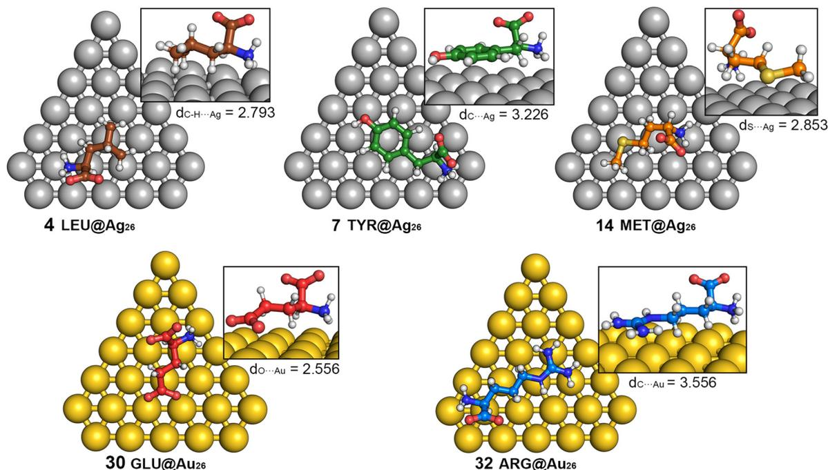
Fig. 2 Optimized geometries at the PBE0-D3/def2-TZVP level of theory of complexes **4**, **7**, **14**, **30** and **32**. The AA...Ag<sub>26</sub>/Au<sub>26</sub> distance is also given in Å.
