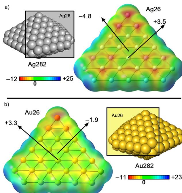
**Fig. 3** MEP surfaces of Ag26 (a) and Au26 (b) layers. The energy values at concrete parts of the surface are given in kcal mol<sup>-1</sup> (0.002 a.u.).
