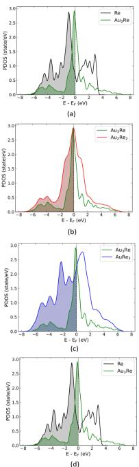
Fig. 7 PDOS of the Re active site in pure Re (001) surfaces (black) and (111) surface alloys; Au@Au<sub>3</sub>Re (green), Au@Au<sub>2</sub>Re<sub>2</sub> (red) and Au@AuRe<sub>3</sub> (blue); (a) Au@Au<sub>3</sub>Re and Re, (b) Au@Au<sub>3</sub>Re and Au@Au<sub>2</sub>Re<sub>2</sub>, (c) Au@Au<sub>3</sub>Re and Au@AuRe3 and (d) Au@AuRe3 and pure Re.
