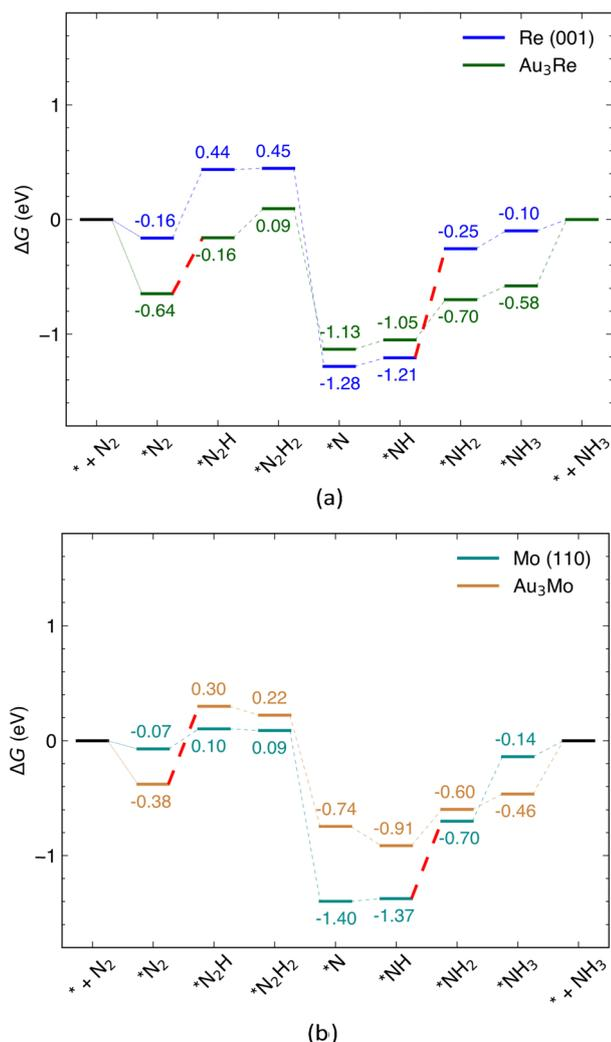
Fig. 6 Free energy profile of the NRR *via* the associative distal mechanism at (a) Re (001) and Au@Au<sub>3</sub>Re (111); (b) Mo (110) and Au@Au<sub>3</sub>Mo (111) surfaces. The PDS which is \*N<sub>2</sub> → \*N<sub>2</sub>H for surface alloys and \*NH → \*NH<sub>2</sub> for pure metal surfaces are shown with dashed red lines.
