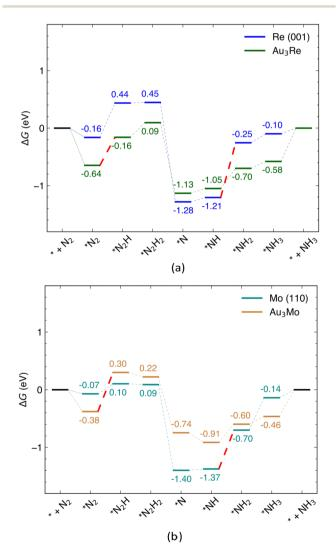
Fig. 6 Free energy profile of the NRR via the associative distal mechanism at (a) Re (001) and  $Au@Au_3Re$  (111); (b) Mo (110) and  $Au@Au_3Mo$  (111) surfaces. The PDS which is  ${}^*N_2 \rightarrow {}^*N_2H$  for surface alloys and  ${}^*NH \rightarrow$ \*NH2 for pure metals surfaces are shown with dashed red lines.
