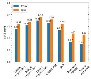
Fig. 2 Training and test prediction accuracy (mean absolute error – MAE) of different MLAs for predicting  $U_{\rm limiting}$  of the NRR at the surface of bimetallic alloy catalysts.
