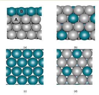
Fig. 1 Bimetallic surface structures considered in the development of the machine learning model. (a) and (c) Side and top view of 111-terminated surface alloy and (b) and (d) side and top view of ordered-intermetallic alloy. A and B (depicted in a) represent metal elements across the periodic
