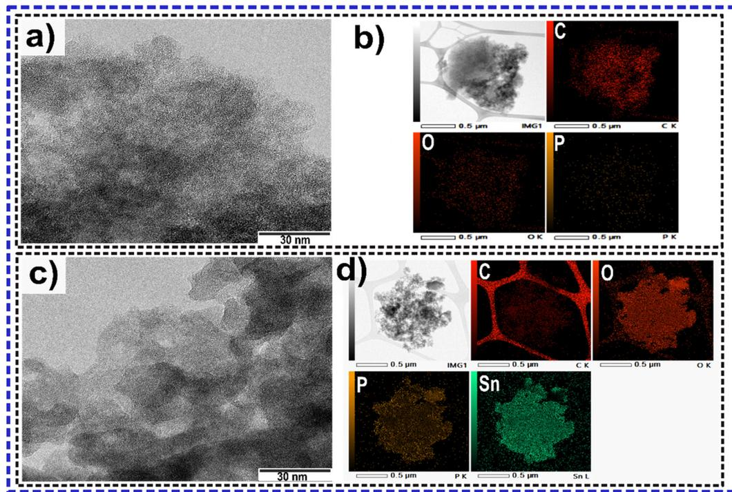
Fig. 2 HRTEM images of (a) BC and (c) BC/SnO<sub>2</sub>, and their corresponding STEM-EDX maps, (b) BC and (d) BC/Sn.
