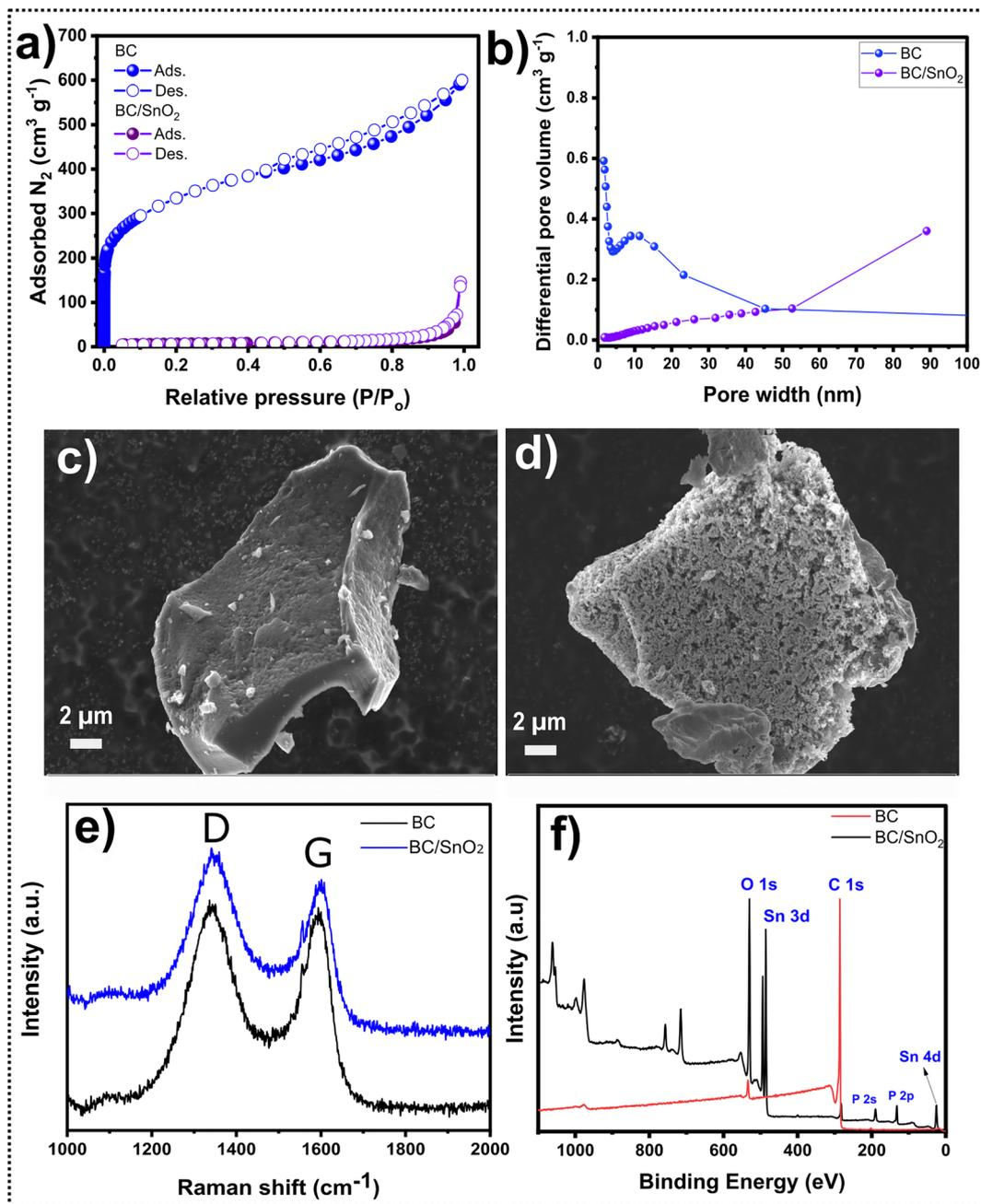
Fig. 1 (a) N<sub>2</sub> isotherms of adsorption–desorption, (b) pore size distribution curves, (c) SEM image of BC at 10k $\times$  magnification, (d) SEM image of BC/SnO<sub>2</sub> at 10k $\times$  magnification, and (e) Raman and (f) XPS spectra of the BC and BC/SnO<sub>2</sub> samples.
