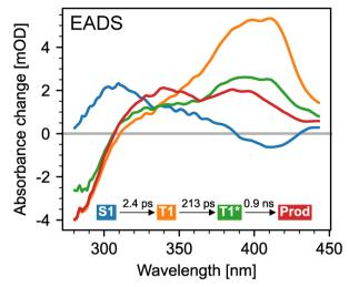
Fig. 4 Spectral components assuming a sequential model for the photochemistry of pHP-FAc in PBS at pH 6.8, upon excitation at 266 nm (see the ESI,† Fig. S9 for a reaction scheme). As only data after 450 fs are used for analysis, the ultrafast transition of the initially excited  $S_2$  to the  $S_1$  is not covered by the model (the S<sub>1</sub> state is reached after fast internal conversion). The colour code is identical for the reaction scheme and the spectral components.
