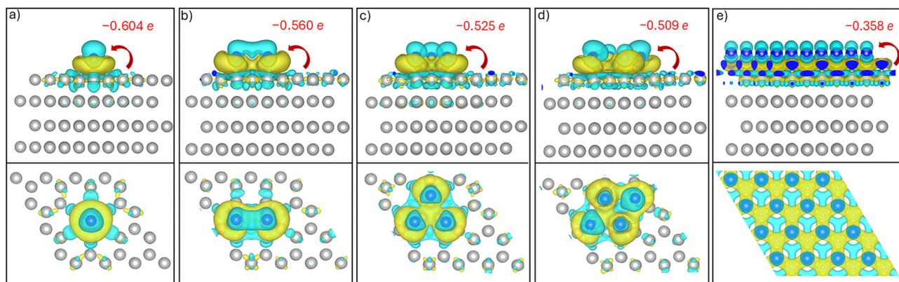
**Fig. 7** Side (top row) and top views (bottom row) of the charge density difference isosurfaces for Ag adatom (a), dimer (b), trimer (c), tetramer (d) and monolayer (e) on the Ti(0001) surface. Values represent the Bader charge gained by one Ag atom in the clusters and monolayer. Electron accumulation and depletion between Ag and Ti atoms are shown in yellow and cyan colors, respectively.
