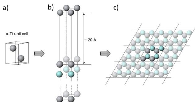
Fig. 1 Bulk and surface slab model of the hcp Ti structure. (a)  $\alpha$ -Ti unit cell of the space group  $P6_3/mmc$ . (b) Side view of the Ti(0001) surface slab model and (c) top view of the bidimensional periodic slab. Gray and pale turquoise spheres represent the surface and subsurface atoms of the Ti slab, respectively.
