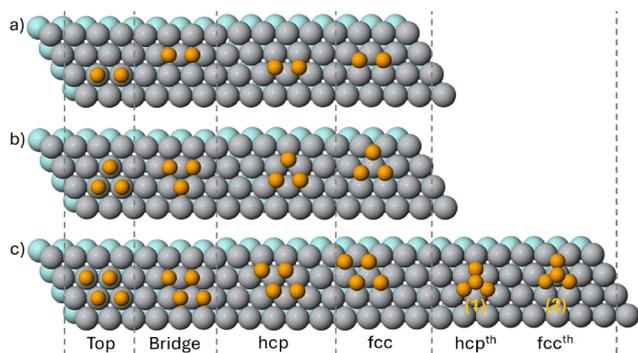
**Fig. 6** Top view of clusters on the Ti(0001) surface at different positions. Rows show the cluster sizes from dimers to tetramers. The orange balls represent the atoms of the cluster. The gray balls show the outermost layer atoms of the substrate. Atoms of the second layer are illustrated by pale turquoise spheres.
