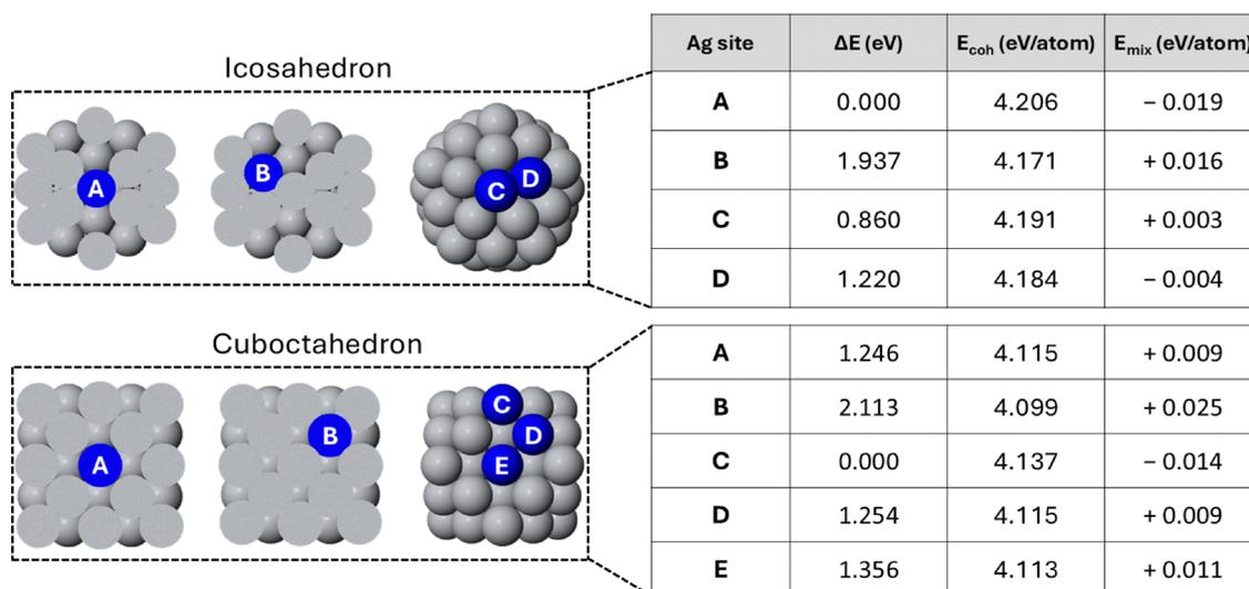
Fig. 2 Site preference of Ag replacing one Ti in the  $\text{Ti}_{55}$  icosahedral (first row) and cuboctahedral (second row) clusters. Blue and gray spheres represent silver and titanium atoms, respectively. Tables show the relative energy differences  $\Delta E$  together with cohesive  $E_{\text{coh}}$  and mixing  $E_{\text{mix}}$  energies. The zero of  $\Delta E$  corresponds to the best position for the Ag impurity in the Ti structure.
