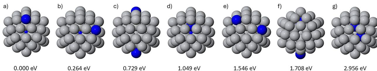
Fig. 3 Configurations (a)–(g) of  $Ti_{53}Ag_2$  in the icosahedral structure, arranged from best (a) to worst (g) in terms of chemical ordering. Titanium atoms are shown in gray and silver atoms in blue. Relative energies of DFT calculations are given. Zero energy corresponds to the lowest placement of Ag atoms in the Ti icosahedron.
