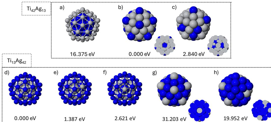
Fig. 4 Optimized homotops of  $\text{Ti}_{42}\text{Ag}_{13}$  (upper panel, (a)–(c)) and  $\text{Ti}_{13}\text{Ag}_{42}$  (lower panel, (d)–(h)). Values represent relative energies of each homotop. Titanium atoms are shown in gray and silver atoms in blue.
