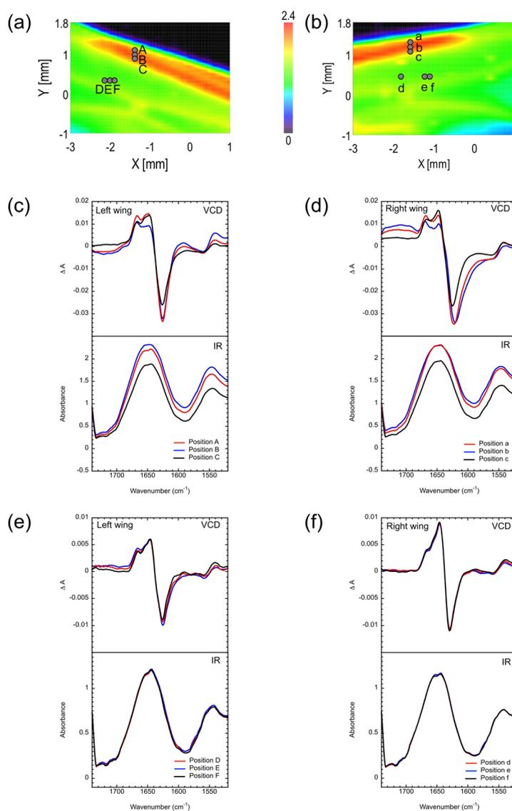
Fig. 4 (a) and (b) IR intensity maps at a fixed wavenumber of  $1650\text{ cm}^{-1}$  of the left (a) and right (b) wings. The analyzed positions are indicated by the filled circles. Positions A–C and a–c are in the near-edge region. Positions D–F and d–f are in the medial region. (c) and (e) VCD and IR spectra obtained from the left wing. (d) and (f) VCD and IR spectra obtained from the right wing.
