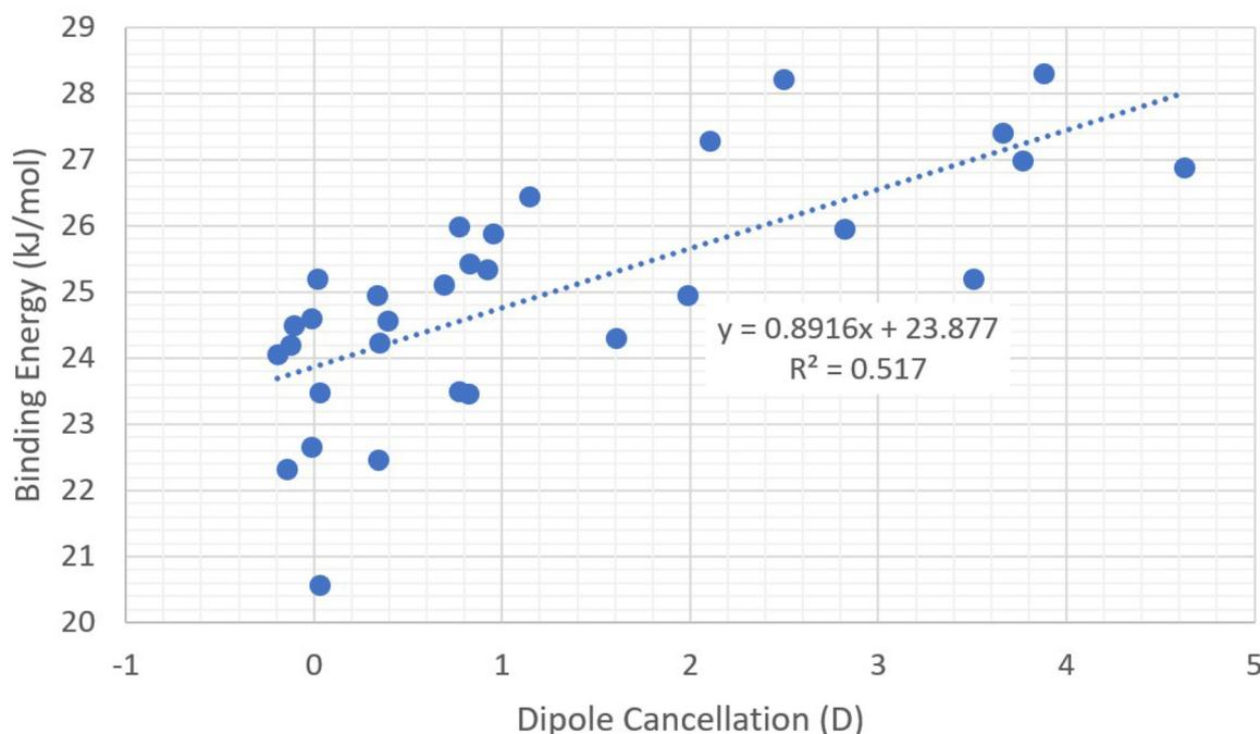
Fig. 5 Scatterplot of  $E_b$  vs. dipole cancellation for all homodimers of Phen and BzQuin, computed at the  $\omega$ B97X-V/def2-QZVPP/SMD(toluene)// $\omega$ B97X-D4/def2-SVP/CPCM(toluene) level of theory. Note that Phen homodimers are capable of negative dipole cancellation when charge transfer between monomers is greater than the original (small) dipoles.
