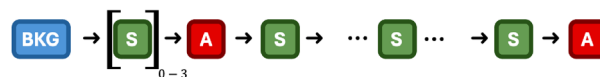
Fig. 10 Proposed scheme for recording a series of FTIR spectra. Blue (BKG) represents the background spectrum, green (S) denotes the proper spectra, and red (A) represents the atmospheric spectra. Measure the first atmospheric spectrum at the beginning (before the proper spectra or after the 1st to 3rd spectrum) and also as the last spectrum of the series. Additional atmospheric spectra can be measured multiple times during the session.
