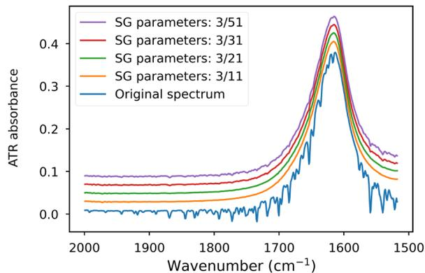
Fig. 3 Influence of Savitzky–Golay smoothing parameters on spectral smoothing in the OH/COO<sup>-</sup> band region of the 10th spectrum of the betaine test set (the same as in Fig. 2).
