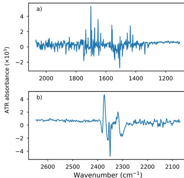
**Fig. 8** Differences between two atmospheric spectra from the betaine spectra test set. Subtraction coefficients were chosen such that the average absorbance value of all points was close to zero. (a) Difference in the amide I band range (as in Fig. 2), (b) difference in the  $\text{CO}_2$  band range. Although both spectra were measured approximately 1 hour apart, complete subtraction of the spectra is not possible.
