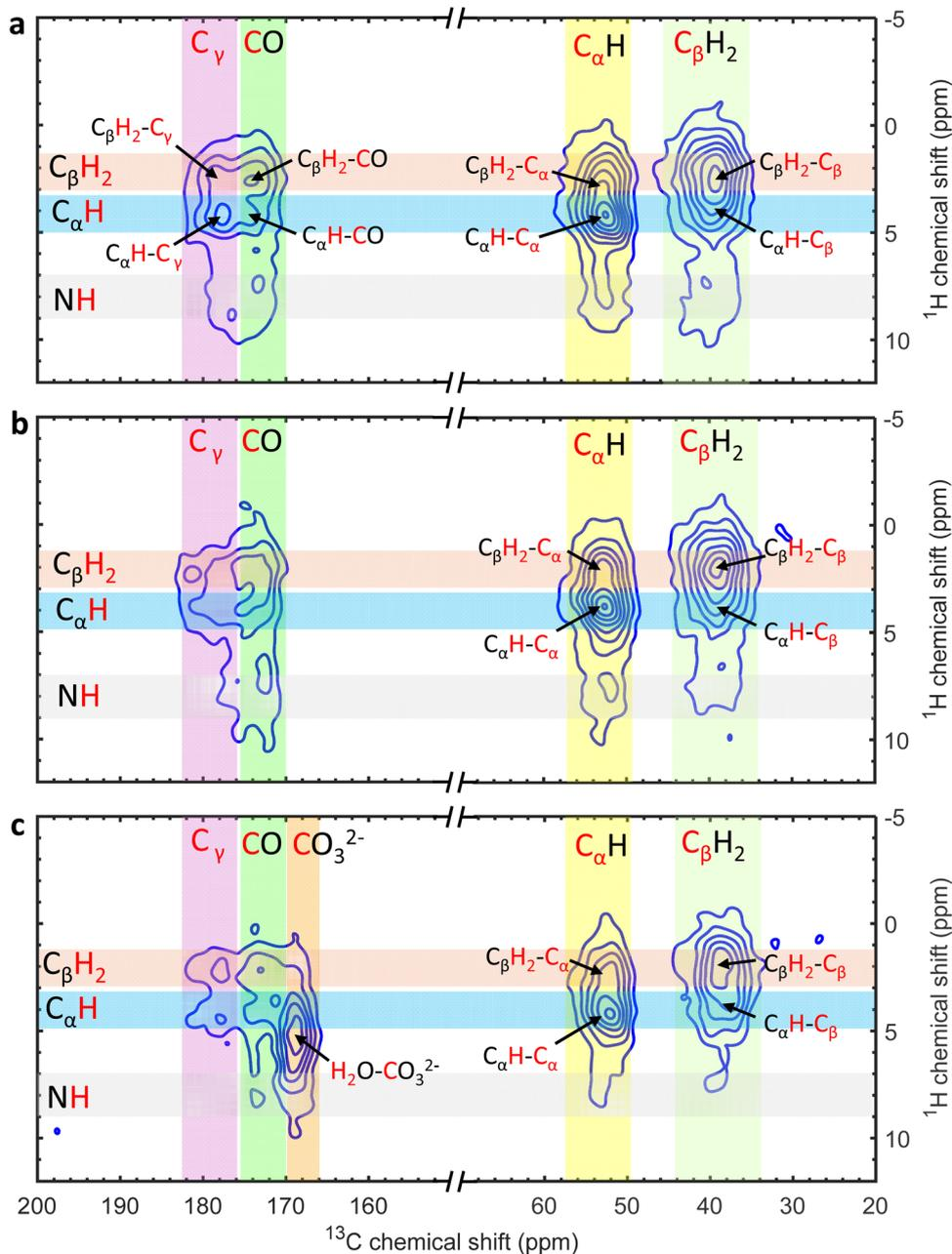
Fig. 2 (a)  $^1\text{H}$ - $^{13}\text{C}$  correlation spectra of (a) PAsp sodium salt, (b) PAsp calcium salt, and (c) PAsp-stabilized disordered ACC. The spinning frequency was 10 kHz. Frequency-switched Lee-Goldburg  $^1\text{H}$ - $^1\text{H}$  decoupling was applied during evolution. Assignments of resolved cross-peaks are indicated.
