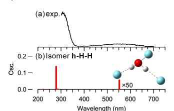
Fig. 3 (a) Observed and (b) calculated spectra of  $(H_2O-Ar_3)^+$  at the EOM-CCSD/aug-cc-pVTZ.
