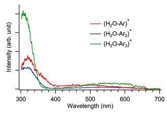
Fig. 4 Comparison among the observed UV-vis spectra of  $(H_2O-Ar_n)^+$ (n = 1-3). These spectra are normalized by the laser power and parent ion intensities
