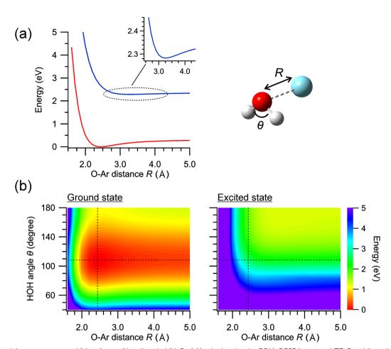
Fig. 7 (a) Potential energy curves and (b) surfaces of hemibonded ( $H_2O-Ar)^+$  calculated at the EOM-CCSD/aug-cc-pVTZ. R and  $\theta$  are defined as shown in the structure of  $(H_2O-Ar)^+$  in the figure. The structural parameters other than R and  $\theta$  were fixed at the equilibrium values obtained from the geometry optimization in the electronic ground state during the calculations
