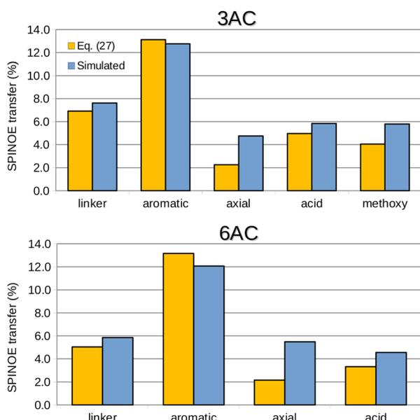
Fig. 8 Maximum SPINOE transfer to the 3AC and 6AC cage protons from hyperpolarised Xe with enhancement factor  $\epsilon_{\text{Xe}} = 1000$ . Simulations that account for proton-proton cross-relaxation are compared to the pseudo two-spin model of eqn (27).
