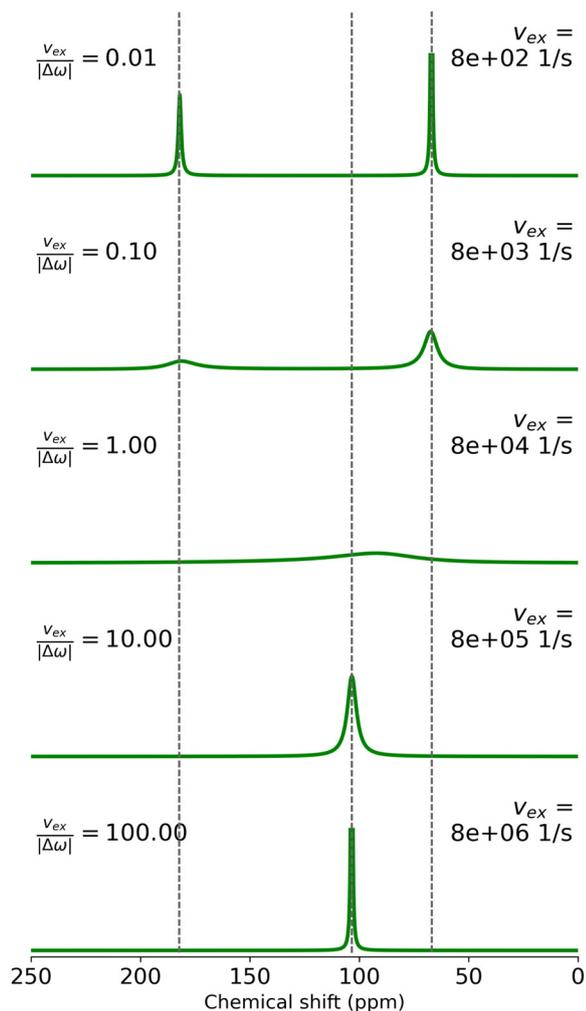
Fig. 11 Simulated NMR spectra of  $^{129}\text{Xe}$  exchanging between free and 6AC-bound environments for different values of exchange rate  $\nu_{\text{ex}}$ . The dashed vertical lines indicate the computed chemical shift values of the free and bound states, as well as their population-weighted average.
