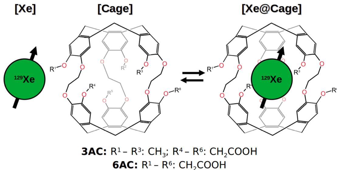
**Fig. 1** Chemical exchange of xenon with a cryptophane cage. The 3AC and 6AC cryptophane-A derivatives studied in the present work are composed of two connected cyclotriphenylene (CTB) bowls. The chemical groups attached to the six binding sites of the cages, R<sup>i</sup> in the figure, are indicated.
