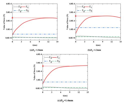
Fig. 11 Forces acting on the particle during the collision of particles with diameters of (a) 1.0 mm, (b) 1.2 mm, and (c) 1.4 mm in the bubble compression phase.
