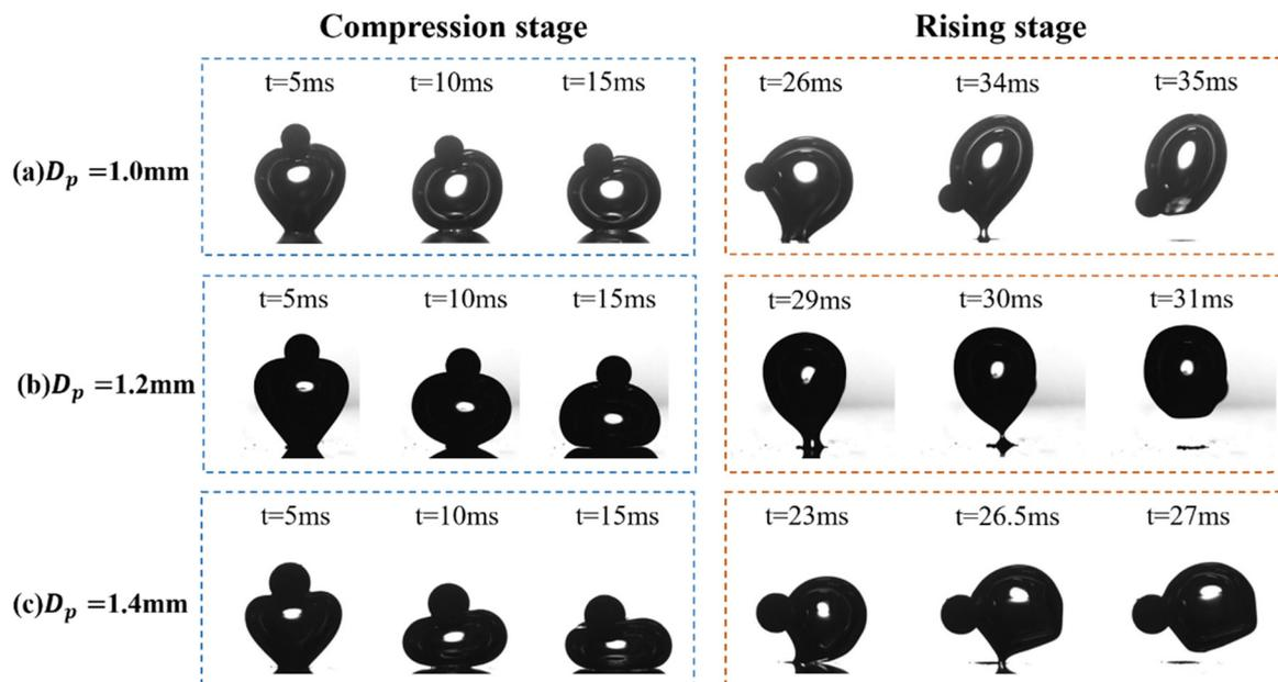
Fig. 10 Trajectory snapshots at different time points for particles with diameters of (a) 1.0 mm, (b) 1.2 mm, and (c) 1.4 mm during collision with a bubble.
