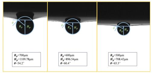
Fig. 2 Measurement of particle contact angle.
