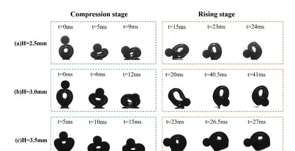
Fig. 7 Snapshots of particle trajectories at different time points during collisions with bubbles of (a) 2.5 mm, (b) 3.0 mm, and (c) 3.5 mm heights.
