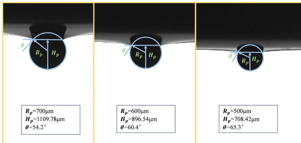
Fig. 2 Measurement of particle contact angle.
