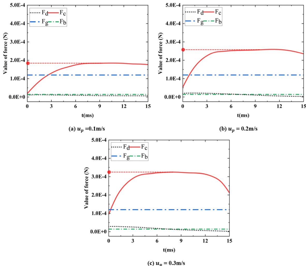
Fig. 5 Forces acting on the bubble during particle-bubble collisions at velocities of (a)  $0.1 \text{ m s}^{-1}$ , (b)  $0.2 \text{ m s}^{-1}$ , and (c)  $0.3 \text{ m s}^{-1}$  in the compression stage.
