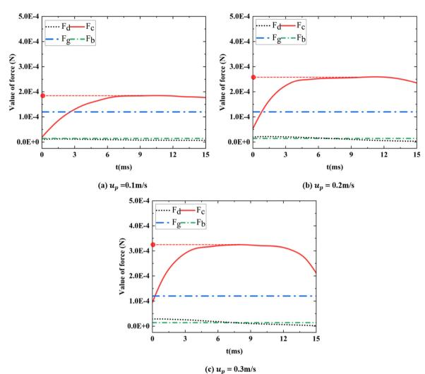
Forces acting on the bubble during particle-bubble collisions at velocities of (a)  $0.1 \,\mathrm{m\,s^{-1}}$ , (b)  $0.2 \,\mathrm{m\,s^{-1}}$ , and (c)  $0.3 \,\mathrm{m\,s^{-1}}$  in the compression stage.
