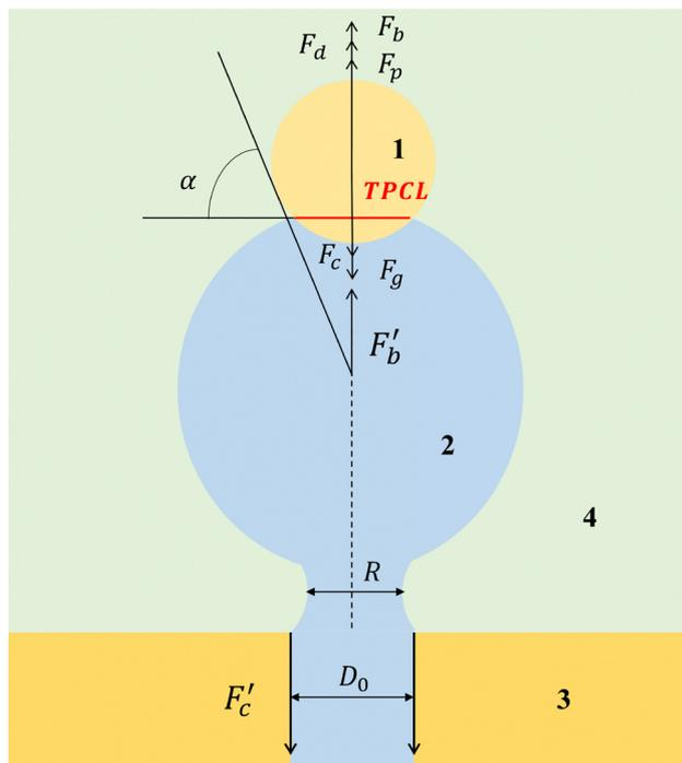
Fig. 3 The forces acting on the particle during the particle–bubble collision process: (1) represents the copper particle, (2) the bubble, (3) the bronze base, and (4) the deionized water.  $\varphi = 0$  (not labeled in the figure).
