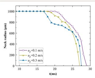
Fig. 6 Change in the bubble neck radius during the rising stage of bubbles.
