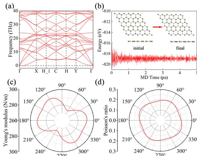
Fig. 2 (a) The phonon dispersion curves, (b) *ab initio* molecular dynamics simulations at 300 K and 5 ps with the free-energy evolution and final structure, (c) Young's modulus, and (d) Poisson's ratio of the  $\text{BC}_2\text{N}$  monolayer.
