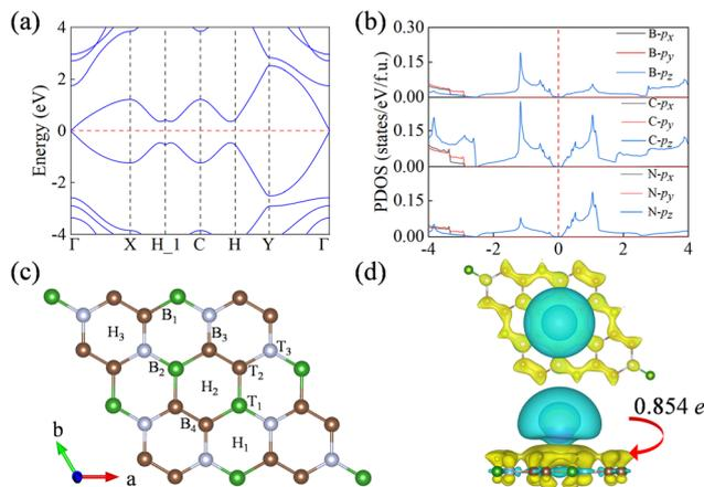
Fig. 3 (a) The electronic band structure and (b) PDOS of the  $\text{BC}_2\text{N}$  monolayer. The Fermi level is set to zero. (c) Top view of the representative adsorption sites on the  $\text{BC}_2\text{N}$  monolayer. (d) Top view and side view of the charge density difference when K is adsorbed on the  $\text{BC}_2\text{N}$  monolayer. Yellow and cyan represent charge accumulation and consumption, respectively.
