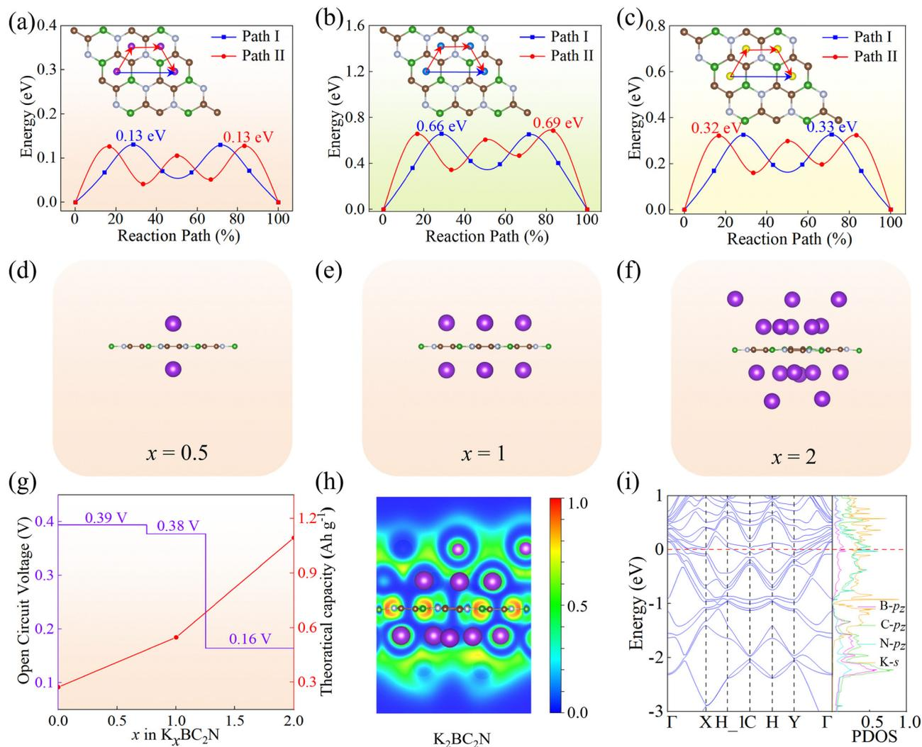
Fig. 4 The diffusion path and diffusion barrier for K (a), Li (b), and Na (c) atoms on the BC<sub>2</sub>N monolayer. (d)–(f) The structures of K atoms adsorbed on the BC<sub>2</sub>N monolayer ( $x$  is the concentration of K ion:  $x = 0.5, 1, 2$ ). (g) The average open circuit voltage (OCV) and theoretical storage capacity (TSC) of the K atom of the BC<sub>2</sub>N monolayer. (h) The electron local function, and (i) the band structures and PDOS of K<sub>2</sub>BC<sub>2</sub>N.
