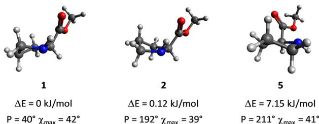
Fig. 3 Optimized structures and relative energies of model conformers of PrOMe at the  $\omega$ B97XD/6-311++G(d,p) level. The pseudorotational phase angle ( $P$ ) and amplitude ( $\chi_{\max}$ ) are described in the Discussion section.
