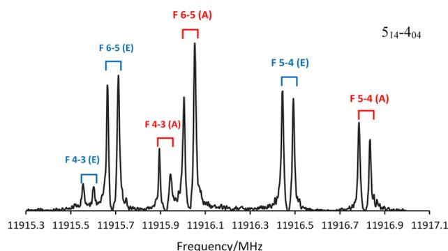
Fig. 2 Portion of the microwave spectrum of PrOMe showing (A) and (E) tunneling state components and nuclear quadrupole hyperfine components of the  $5_{15}-4_{04}$  rotational transition with 25 free induction decays averaged.
