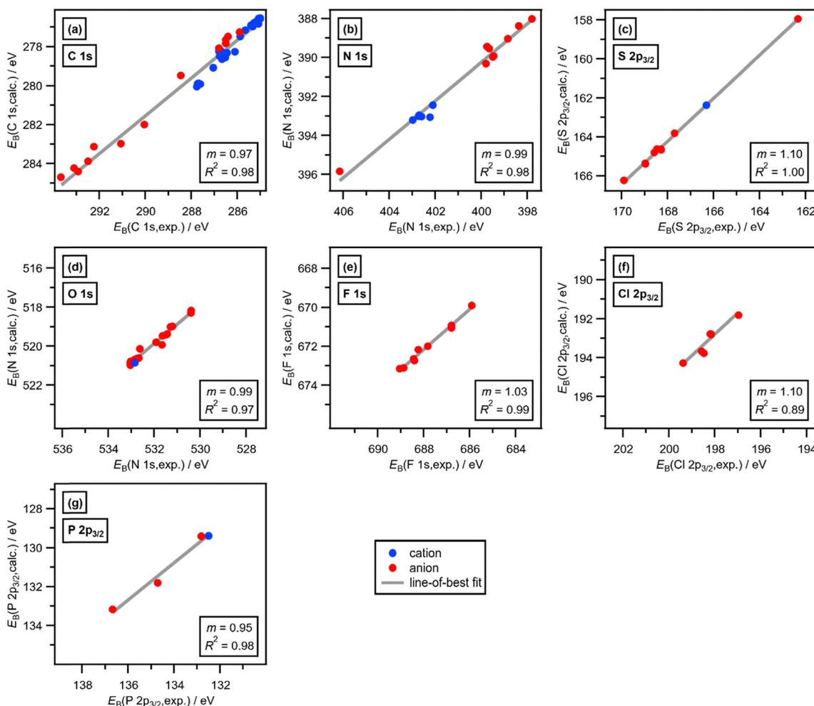
Fig. 1 Calculated binding energy,  $E_B(\text{calc.})$  from lone-ion-SMD against experimental XPS binding energy,  $E_B(\text{exp.})$  for: (a) C 1s, (b) N 1s, (c) S 2p<sub>3/2</sub>, (d) O 1s, (e) F 1s, (f) Cl 2p<sub>3/2</sub>, (g) P 2p<sub>3/2</sub>.  $m$  is the gradient of each line-of-best fit. The experimental uncertainty is  $\pm 0.10$  eV; the calculated uncertainty is  $\pm 0.20$  eV.
