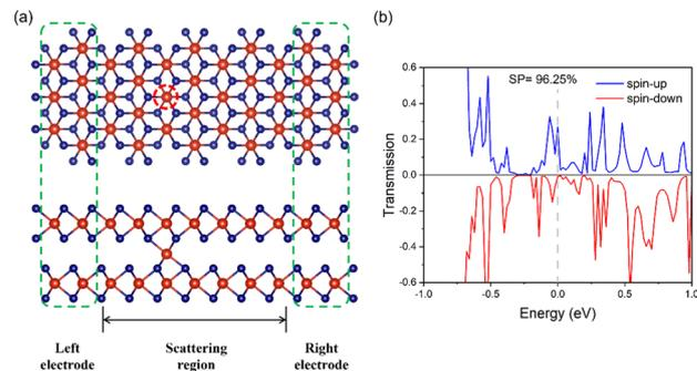
Fig. 5 (a) Schematic diagram of the dual-probe transport device for spin transport calculations, including the semi-infinite left and right electrodes (in dashed) and the central device region. (b) Spin-polarized transmission spectrum of the device at a bias voltage of 0.2 V.
