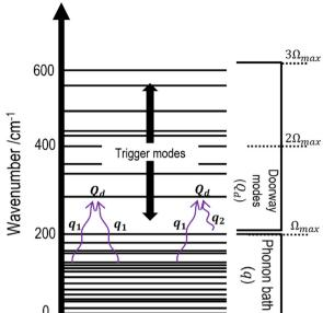
Fig. 3 Schematic diagram illustrating the vibrational up-pumping process.
