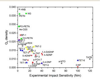
Fig. 6 Doorway density versus experimental impact sensitivity. Colour scheme relates to compound classes shown in Fig. 2.
