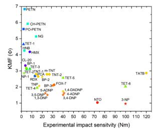
Fig. 7 KMF vs. experimental impact sensitivities for the compounds included in the vibrational up-pumping study, colour coded according to the number of trigger bonds ( $N_{\text{trig}}$ , red – low, blue – high) per molecule.
