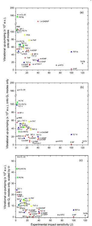
Fig. 5 Vibrational up-pumping densities vs. experimental impact sensitivity values (a) projected onto all molecular vibrations that fall between  $1-3\Omega_{max}$ , and (b) only those molecular vibrations that contain weak bond stretch character, and (c) further scaled according to weak bond strengths. Colour scheme relates to compound classes shown in Fig. 2. Experimental impact sensitivities are taken from ref. 27 and 41–57.
