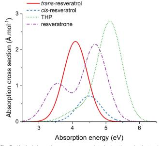
Fig. 3 Vertical absorption spectrum convoluted using the main electronic transitions for trans-resveratrol, cis-resveratrol, THP and resveratrone.
