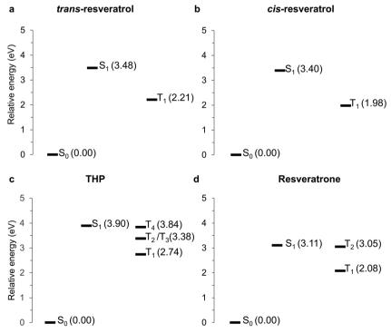
Fig. 4 Schematic energy diagram (considering microsolvation) for (a) trans-resveratrol, (b) cis-resveratrol, (c) THP, and (d) resveratrone showing the energies of the singlet and triplet states at their respective optimized geometries. The energy values are relative to the S<sub>0</sub> minimum.
