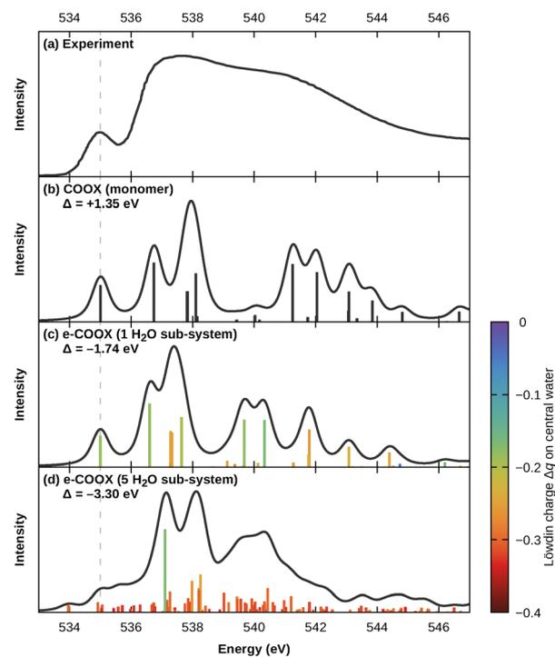
**Fig. 6** (a) Experimental and (b)–(d) computed X-ray absorption spectra of liquid water. The experimental spectrum is adapted from ref. 65 and computed spectra are obtained using e-COOX@PBE0/aug-pcX-2/aug-pcseg-2/pcseg-2 (see the text for further details). Line spectra broadened with Voigt profiles with a HWHM of 0.2 eV for both Gaussian and Lorentzian components.
