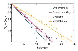
Fig. 4 Plot of the transient amplitude signals for all samples (cytochrome c, myoglobin in H<sub>2</sub>O and D<sub>2</sub>O) and the fits obtained via egn (1). Data and fit were linearized with eqn (2) and the semi-logarithmic scale of the plot.
