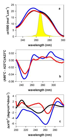
Fig. 1 Comparison of the steady-state absorption (a), thermal (b) and CD spectra (c) of GT (red) and TG (blue) and an equimolar mixture of dG and dT (black). In (a) the absorbance is normalized at 266 nm, corresponding to the peak intensity of the exciting laser pulse (yellow). The thermal spectra are the difference between the steady-state absorption spectra recorded for each dinucleotide at 95 °C (A95 °C) and 23 °C (A23 °C), divided by A23 °C.
