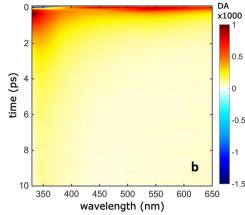
Contour 2D maps recorded for GT (a) and an equimolar mixture of dG and dT (b) with excitation at 266 nm
