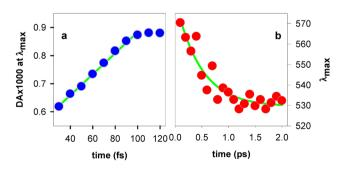
Fig. 11 Variation of the peak intensity at the 430-450 nm spectral domain (a) and position of the maximum of the long wavelength band (b) observed in the GT TAS. Green lines are fits with linear (a) and monoexponential (b) functions.
