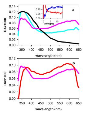
Fig. 9 (a) TAS recorded for dT at 2.5 ps (pink) and 40 ps (cyan); the TMP TAS recorded at 200 ns by ns TA spectroscopy following 266 nm excitation is shown in black.  $^{48}$  Inset: TA signals of dT at 350 nm (blue) and 600 nm (red). (b) Comparison between the TAS of GT at 40 ps (red) and that of dT at 2.5 ps (pink).
