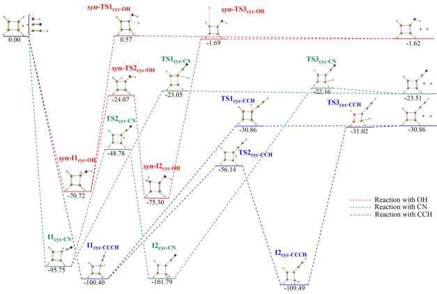
Fig. 4 Relative energies (in kcal mol<sup>-1</sup>) for the stationary points located along the gas phase reaction of cyclobutadiene with hydroxyl, cyano, and ethynyl radicals computed at the CCSD(T)-F12/cc-pVTZ-F12//B2PLYPD3/aug-cc-pVTZ level. ZPV energies are included.
