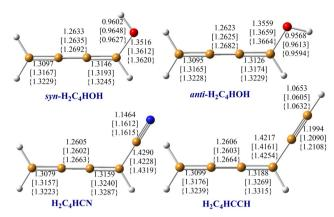
Fig. 2 Geometrical parameters of the butatriene derivates, H2CCCCHX with X = OH, CN, and CCH, calculated at the M08HX/aug-cc-pVTZ, B2PLYPD3/aug-cc-pVTZ (in brackets) and CCSD(T)-F12/cc-pVTZ-F12 (in curly bracket) levels. Distances are given in Angstroms.
