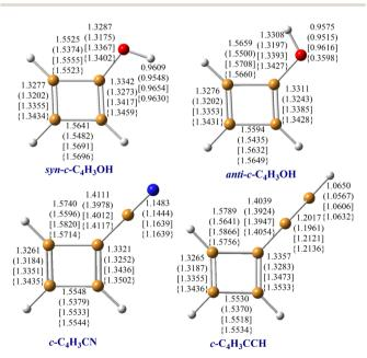
Fig. 1 Geometrical parameters of the cyclobutadiene derivates,  $c-C_4H_3X$ with X = OH, CN, and CCH, calculated at the M08HX/aug-cc-pVTZ, MPWB1K/aug-cc-pVTZ (in parentheses), B2PLYPD3/aug-cc-pVTZ (in brackets) and CCSD(T)-F12/cc-pVTZ-F12 (in curly bracket) levels. Distances are given in Angstroms.
