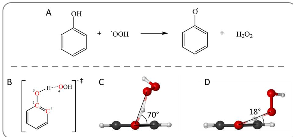
Fig. 1 (A) Hydrogen abstraction from phenol by a hydroperoxyl radical. (B) Structure of the transition state for the hydrogen abstraction from phenol by  $\bullet\text{OOH}$ . The C–C–O–O dihedral angle is highlighted by red labels. (C) Optimized structures of the relaxed structure with a C–C–O–O dihedral angle of  $70^\circ$  and (D) of the partially constrained structure with a C–C–O–O dihedral angle of  $18^\circ$ . Level of theory: M06-2X/6-31G(d).
