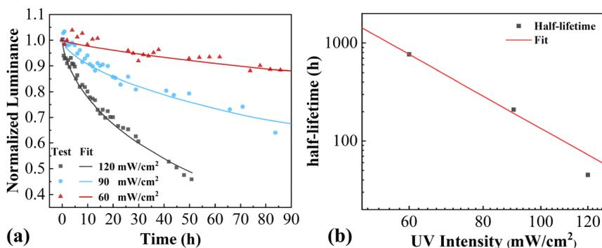
Fig. 4 (a) SED model of  $L$ - $T$  characteristics under UV irradiances of 60, 90, and 120 mW cm<sup>-2</sup>. (b) The relationship between UV intensity and half-lifetime of device D1.
