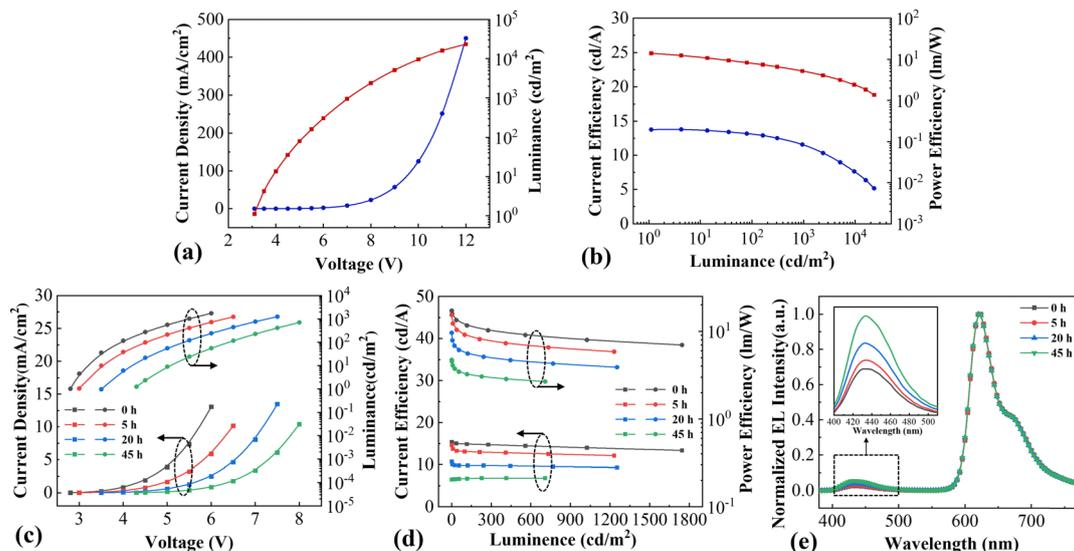
Fig. 2 (a)  $J$ - $V$ - $L$  and (b)  $L$ - $CE$ - $PE$  of pristine device D1. (c)  $J$ - $V$ - $L$ , (d)  $L$ - $CE$ - $PE$ , and (e) EL spectra of device D1 at initial state, 5 h, 20 h, and 45 h under  $120 \text{ mW cm}^{-2}$  UV irradiance.
