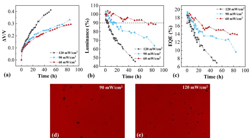
Fig. 3 (a)  $V$ - $T$ , (b)  $L$ - $T$ , and (c)  $EQE$ - $T$  characteristics of device D1 at UV irradiances of  $60$ ,  $90$ , and  $120 \text{ mW cm}^{-2}$  at  $10 \text{ mA cm}^{-2}$ . Microscopic images of device D1 after 50 h of UV irradiances at (d)  $90 \text{ mW cm}^{-2}$  and (e)  $120 \text{ mW cm}^{-2}$ .
