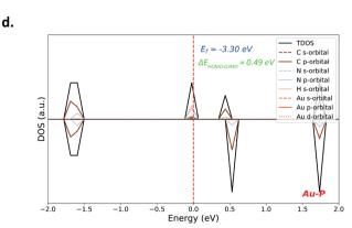
Fig. 2 Total and partial DOS plots of molecules. (a) Free-based (2H-P) (b) Cu doped (Cu-P) (c) Ag doped (Ag-P) and (d) Au doped (Au-P). Fermi level is shown by the dotted vertical lines set to 0 eV.
