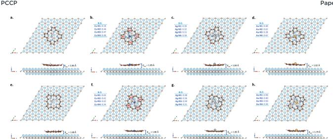
Fig. 4 Adsorption of bare/doped porphine molecules on Ti<sub>2</sub>C surface. (a) – (d) 2H-P, Cu-P, Aq-P, and Au-P for model-I, respectively. (e) – (h) 2H-P, Cu-P, Aq-P, and Au-P for model-II, respectively. Bond order (BO) values of the metal atoms are given as insets
