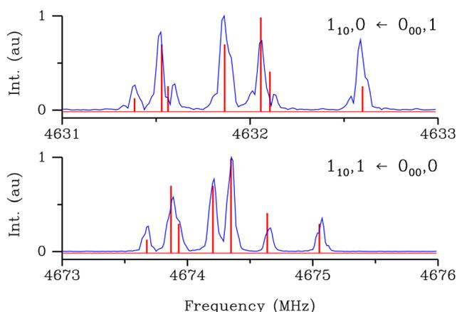
Fig. 5 Comparisons between the observed spectrum and a calculated stick spectrum for the  $1_{10}$ ,  $1 \leftarrow 0_{00}$ ,  $0$  and  $1_{10}$ ,  $0 \leftarrow 0_{00}$ ,  $1$  transitions. Both spectra are plotted as a function of the frequency in MHz. The lists of predicted hyperfine transitions are given in Table S2 of the ESI.<sup>†</sup>
