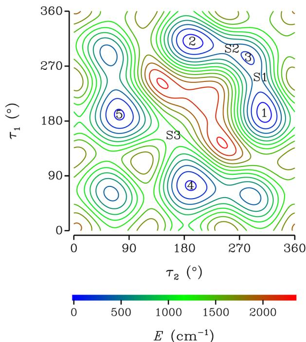
Fig. 2 The relaxed two-dimensional potential energy surface of CDA as a function of the dihedral angles  $\tau_1$  and  $\tau_2$ . Contour lines corresponding to equally spaced energy values with a spacing of 200  $cm^{-1}$  are drawn from 100 to 2300  $cm^{-1}$ . 5 minima numbered 1 through 5; and 3 saddle points labeled S1, S2, and S3 can be seen.
