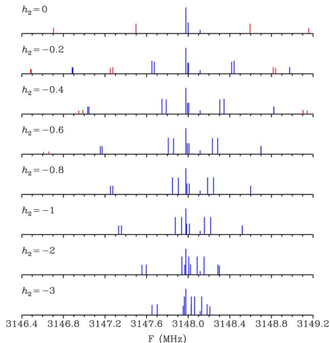
Fig. 4 Calculated stick spectra of the hyperfine structure of the two tunneling components of the  $1_{01} \leftarrow 0_{00}$  transitions for values of the tunneling parameter  $h_2$  ranging from 0 to  $-3$  MHz. Hyperfine components are drawn in blue (red) for  $\Delta l$  even (odd).
