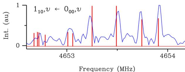
Fig. 6 Comparisons between the observed spectrum and a calculated stick spectrum, plotted as a function of the frequency in MHz, for the hyperfine structure of the transitions  $1_{10}, \nu \leftarrow 0_{00}, \nu$ , with  $\nu = 0$  and 1. These transitions being forbidden, their hyperfine components gain strength through mixings due to the hyperfine coupling Hamiltonian. The lists of predicted hyperfine transitions are given in Table S2 of the ESI.<sup>†</sup>
