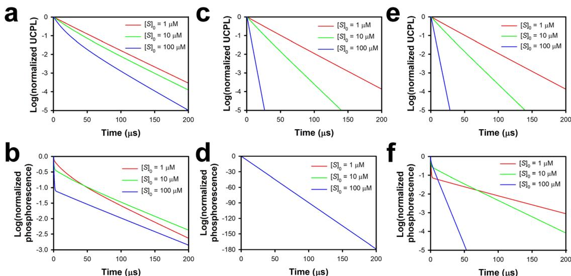
Fig. 5 Transient decays derived from kinetic models including: (a) upconverted fluorescence in the presence of reverse TET only; (b) phosphorescence in the presence of reverse TET only; (c) upconverted fluorescence in the presence of dynamic quenching only; (d) phosphorescence in the presence of dynamic quenching only; (e) upconverted fluorescence in the presence of both reverse TET and dynamic quenching; and (f) phosphorescence in the presence of both reverse TET and dynamic quenching.
