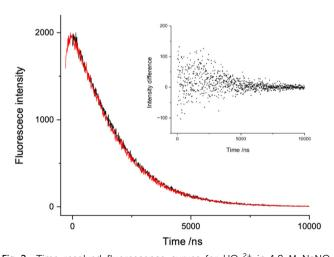
Fig. 2 Time-resolved fluorescence curves for UO<sub>2</sub><sup>2+</sup> in 1.8 M NaNO<sub>3</sub> solution. The red and black curves correspond to fluorescence detection at 500 and 510 nm. The inset shows the difference between these curves.
