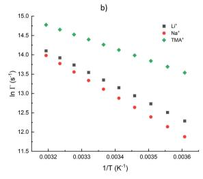
Fig. 5 Fluorescence decay rates as a function of temperature. (a) Measurements were carried out in H<sub>2</sub>O with added nitrate salt concentrations of 1.8 M. (b) Measurements were carried out in D<sub>2</sub>O with added nitrate salt concentrations of 1.8 M.
