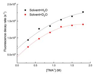
Fig. 7 Decay rate vs. TMA+ concentration for uranyl fluorescence from H<sub>2</sub>O and D<sub>2</sub>O solutions. Measurements taken at 20 °C.
