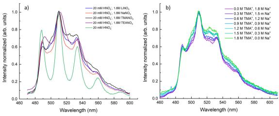
Fig. 1 Steady-state emission spectra of uranyl from 460-600 nm. (a) The emission from solutions containing Li<sup>+</sup>, Na<sup>+</sup>, TMA<sup>+</sup>, and TEA<sup>+</sup> nitrate salts are compared to uranyl nitrate in nitric acid. (b) Change in emission bands as NaNO3 is replaced with TMANO3. Excitation wavelength was 394 nm for all samples.
