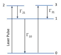
Fig. 8 Proposed energy level scheme for the non-exponential fluorescence decay of uranyl. See text for details
