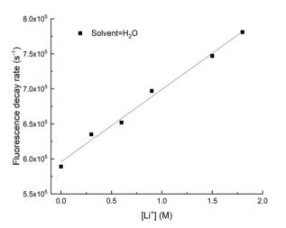
Fig. 6 Decay rate vs. Li<sup>+</sup> concentration for uranyl fluorescence from H<sub>2</sub>O solutions. Measurements taken at 20 °C.
