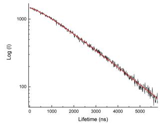
Fig. 3 Semi-log plot of the time-resolved fluorescence from a uranyl solution that contained 1.8 M NaNO3 at 20 °C.
