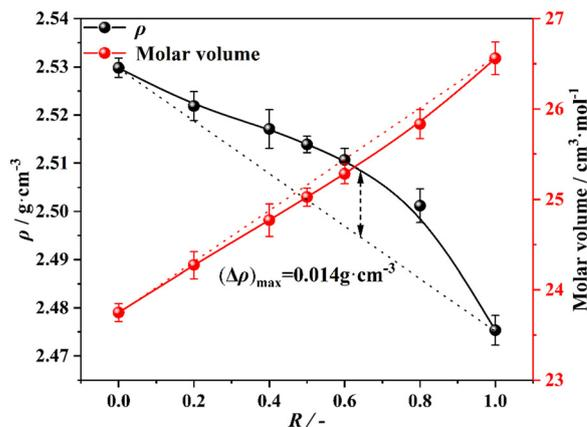
Fig. 5 Compositional dependence of the density ( $\rho$ ) and molar volume of the  $65.0\text{SiO}_2 \cdot 5.0\text{B}_2\text{O}_3 \cdot (17.6 - x)\text{Na}_2\text{O} \cdot x\text{K}_2\text{O} \cdot 7.5\text{CaO} \cdot 4.9\text{MgO}$  glasses as a function of different molar ratios  $R$ , where  $R$  is equal to the molar ratio of  $[\text{K}_2\text{O}]/([\text{Na}_2\text{O}] + [\text{K}_2\text{O}])$ . The dashed line is a guide for the eye.
