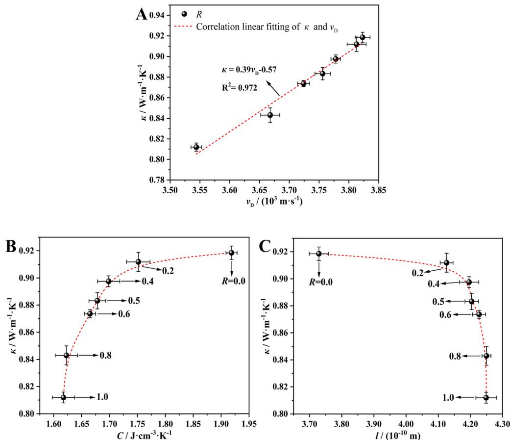
Fig. 3 Relationship between thermal conductivity ( $\kappa$ ) and (A) Debye sound velocity ( $\nu_D$ ), (B) volumetric heat capacity ( $C$ ) and (C) phonon mean free path ( $l$ ) for the glasses with different  $R$  investigated in this work. The dashed line is a guide for the eye.
