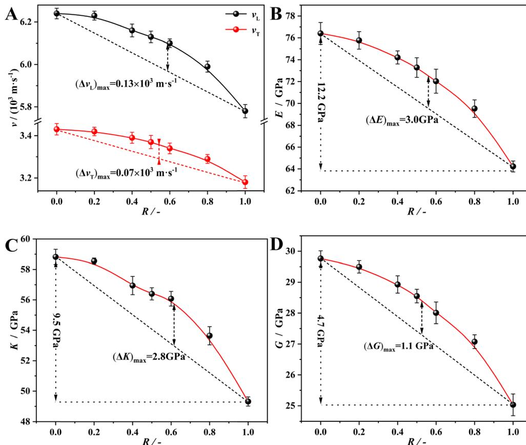
Fig. 4 Compositional dependence of (A) longitudinal sound velocity ( $\nu_L$ ) and transversal sound velocity ( $\nu_T$ ), (B) Young's modulus  $E$ , (C) Bulk modulus  $K$  and (D) Shear modulus  $G$  at room temperature as a function of the molar ratio  $R$  ( $R$  is equal to the molar ratio of  $[\text{K}_2\text{O}]/([\text{Na}_2\text{O}] + [\text{K}_2\text{O}])$ ).
