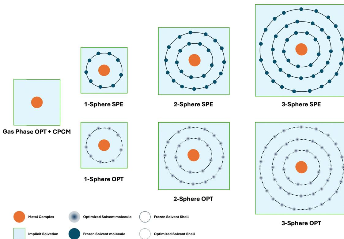
**Scheme 1** Schematic overview of the three-layer micro-solvation model. Each step corresponds to the solvation procedure described in Table 1, where successive layers of explicit water molecules are added around the Fe complex. Optimization (OPT) and single-point energy (SPE) calculations are performed at each stage (1,2,3) to refine solute–solvent interactions.
