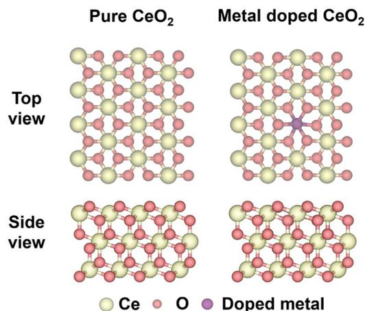
Fig. 1 Structural diagrams of pure CeO<sub>2</sub> and metal-doped CeO<sub>2</sub>.
