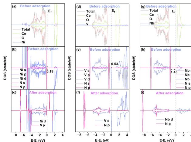
Fig. 6 Partial density of electronic state for N of  $\text{NH}_3$  and metal-doped  $\text{CeO}_2$  before and after  $\text{NH}_3$  adsorption. (a)–(c) Ni-doped, (d)–(f) V-doped and (g)–(i) Nb-doped  $\text{CeO}_2$ . The Fermi level (dashed line) has been set at 0 eV.
