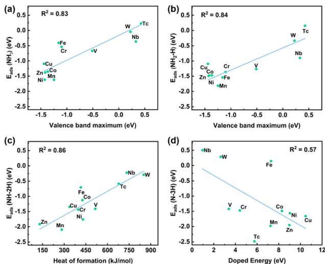
Fig. 5 (a) and (b) Valence band maximum, (c) heat of formation, and (d) doped energy of metal dopant as functions of the adsorption energies of (a)  $\text{NH}_3$ , (b)  $\text{NH}_2\text{-H}$ , (c)  $\text{NH-2H}$  and (d)  $\text{N-3H}$  species in  $\text{NH}_3$  dissociation.
