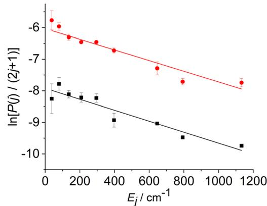
Fig. 4 Boltzmann plot for CN ( $X^2\Sigma^+$ ) scattered from squalane (black) and PFPE (red) surfaces, spanning rotational levels in the  $f_1$  spin-rotation manifold ranging from  $j = 4.5$  to  $j = 24.5$  together with the linear best fit.
