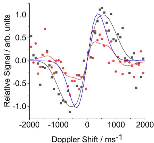
Fig. 5 FM absorption (black) and dispersion (red) Doppler line shapes for CN scattering from a squalane surface into  $j = 12.5$  integrated from  $176$  to  $266 \mu\text{s}$ . Experimental data are shown by the squares/circles and the black and red lines indicate the respective fits. The blue line shows the simulated FM absorption line shape for a Maxwell-Boltzmann distribution of CN at  $298 \text{ K}$ .
