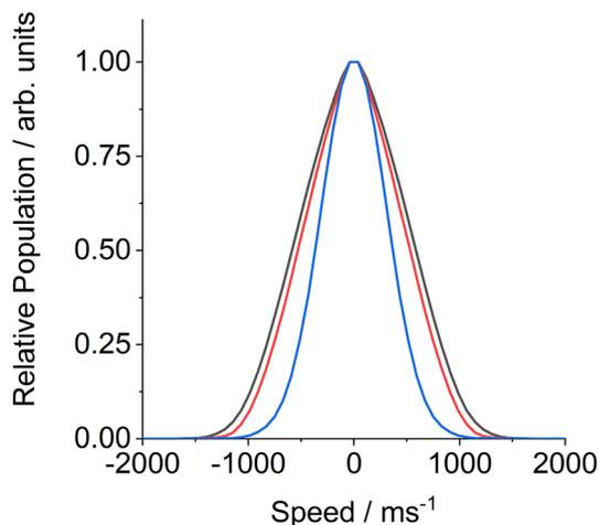
Fig. 6 Speed distributions of CN radicals, perpendicular to the surface normal, after scattering from a squalane (black) and PFPE (red) surface into  $j = 12.5$ . The squalane distribution was determined from the fit to the data shown in Fig. 5. The blue line shows the (Gaussian) 1-d speed distribution of a 298 K Maxwell–Boltzmann distribution of CN.
