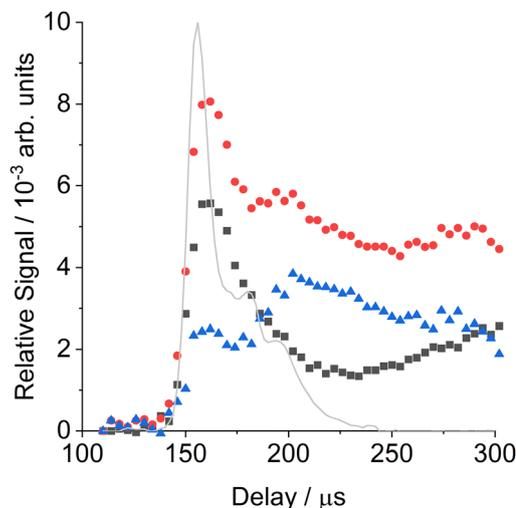
Fig. 2 Appearance profiles for  $j = 12.5$  for wheel-out (black squares) and wheel-in (red circles) and the difference (blue triangles), representing relative population as a function of discharge-probe delay. The solid grey line shows the appearance profile of  $j = 0.5$  for the incident CN (multiplied by a factor of 0.01).
