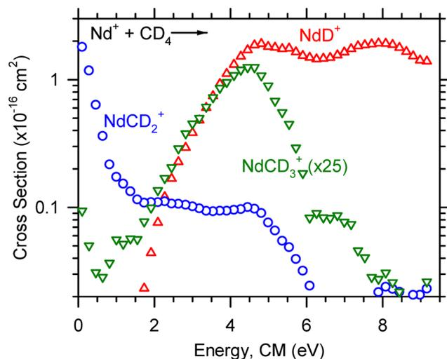
Fig. 3 Product ion cross sections for the reaction of  $\text{Nd}^+ + \text{CD}_4$  as a function of ion kinetic energy in the center-of-mass frame,  $E_{\text{CM}}$ . The dominant product at low energies is  $\text{NdCD}_2^+$  (blue circle). At higher energies the dominant product is  $\text{NdD}^+$  (red triangle). Minor product  $\text{CeCD}_3^+$  (green inverted triangle) is also observed. This channel has been magnified as indicated.
