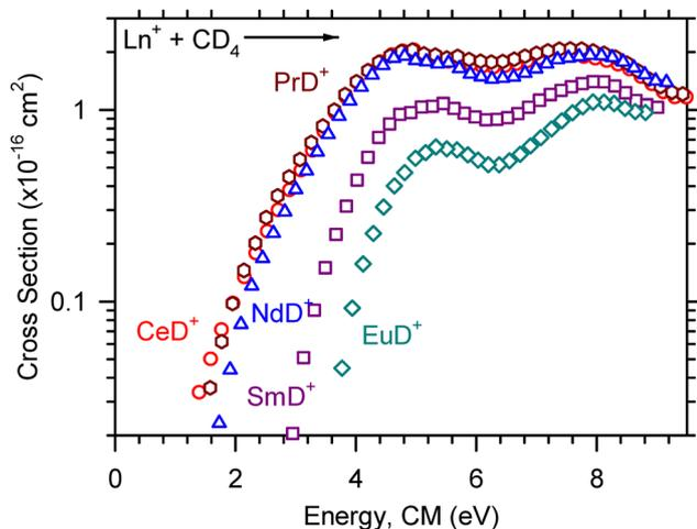
Fig. 6 LnD<sup>+</sup> product ion cross sections for the reaction of Ln<sup>+</sup> + CD<sub>4</sub> → LnD<sup>+</sup> + CD<sub>3</sub> as a function of ion kinetic energy in the center-of-mass frame, *E*<sub>CM</sub>. The observed apparent thresholds are CeD<sup>+</sup> (red circle) ≥ PrD<sup>+</sup> (dark red hexagon) > NdD<sup>+</sup> (blue triangle) > SmD<sup>+</sup> (purple square) > EuD<sup>+</sup> (teal diamond).
