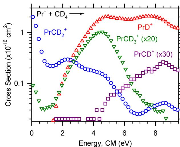
Fig. 2 Product ion cross sections for the reaction of  $\text{Pr}^+ + \text{CD}_4$  as a function of ion kinetic energy in the center-of-mass frame,  $E_{\text{CM}}$ . The dominant product at low energies is  $\text{PrCD}_2^+$  (blue circle). At higher energies the dominant product is  $\text{PrD}^+$  (red triangle). Minor products  $\text{PrCD}_3^+$  (green inverted triangle) and  $\text{PrCD}^+$  (purple square) are also observed. These channels have been magnified as indicated.
