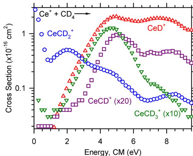
Fig. 1 Product ion cross sections for the reaction of  $\text{Ce}^+ + \text{CD}_4$  as a function of ion kinetic energy in the center-of-mass frame,  $E_{\text{CM}}$ . The dominant product at low energies is  $\text{CeCD}_2^+$  (blue circle). At higher energies the dominant product is  $\text{CeD}^+$  (red triangle). Minor products  $\text{CeCD}_3^+$  (green inverted triangle) and  $\text{CeCD}^+$  (purple square) are also observed. These channels have been magnified as indicated.
