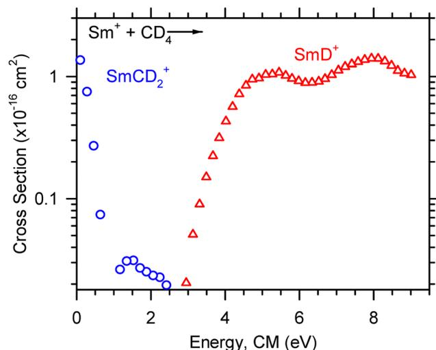
Fig. 4 Product ion cross sections for the reaction of  $\text{Sm}^+ + \text{CD}_4$  as a function of ion kinetic energy in the center-of-mass frame,  $E_{\text{CM}}$ . The dominant product at low energies is  $\text{SmCD}_2^+$  (blue circle). At higher energies the dominant product is  $\text{SmD}^+$  (red triangle).
