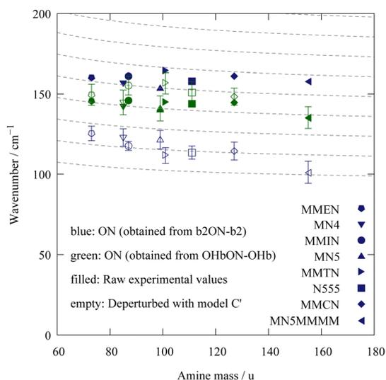
**Fig. 8** Trend of the dimer ON stretching vibration on top of b2 excitation (blue) and on top of OHb excitation (green) with the mass of the amine. The dashed curves indicate the kinematic trend expected from the reduced mass, if the force constant remains constant. Shown are the values obtained from the difference of the raw experimental band positions (filled symbols) and values after deperturbation of the resonances based on model C'. See text for explanations.
