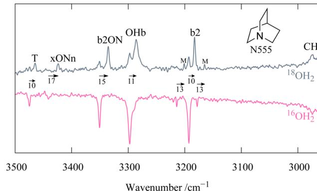
Fig. 5 Comparison of the OH stretching spectrum of N555 with <sup>16</sup>OH<sub>2</sub> (bottom, inverted) to the same spectrum enriched in <sup>18</sup>OH<sub>2</sub>. The 16–18-isotope shifts in cm<sup>-1</sup> are clarified by arrows (see Table S15 in the ESI,<sup>†</sup> for details).
