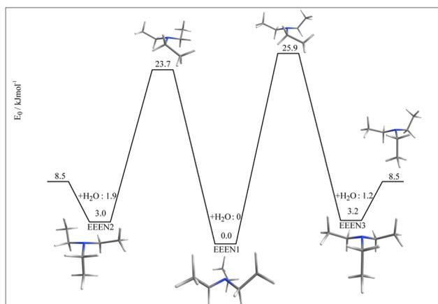
**Fig. 9** The two most stable excited conformers of EEEN (EEEN2, EEEN3) separated by high barriers from the global minimum (EEEN1) but by a lower barrier from each other. Given are relative energies for the monomers as well as for the water complexes, in kJ mol<sup>−1</sup>. The jet spectra are expected to represent a mix of EEEN1 and EEEN2 and/or EEEN3.
