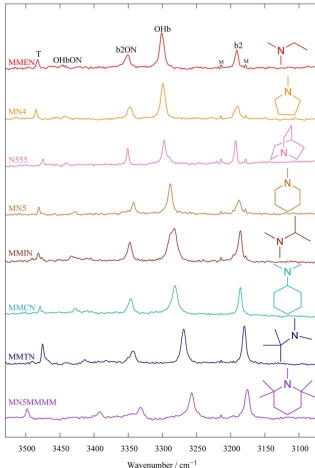
**Fig. 12** Spectra of the 8 amine mono- and dihydrates to be included into the HyDRA database, sorted by decreasing deperturbed (and also dominant signal) OHb wavenumber. The sorting corresponds to increasing  $n_{\beta}-n_r$  value (see text). b2 and b2ON show no clear trend, whereas the weakest signal follows the OHb trend, supporting its OHbON assignment. T is assigned to the indirectly amine-coordinating OHb of the dihydrate and shows an opposite trend for the lowest trace.
