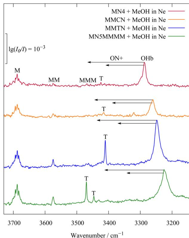
Fig. 11 Spectra for methanol complexes of four tertiary amines, with strong  $OHb$  stretching signals from monomethanolates besides dimethanolates (T) and methanol (M) homodimers (MM) and - trimers (MMM). Arrows indicate where bands with  $OHbON$  character would be expected in an ( $ON$  unscaled) harmonic DFT picture (two monomethanolate vibrations carry significant  $ON$  stretching character).
