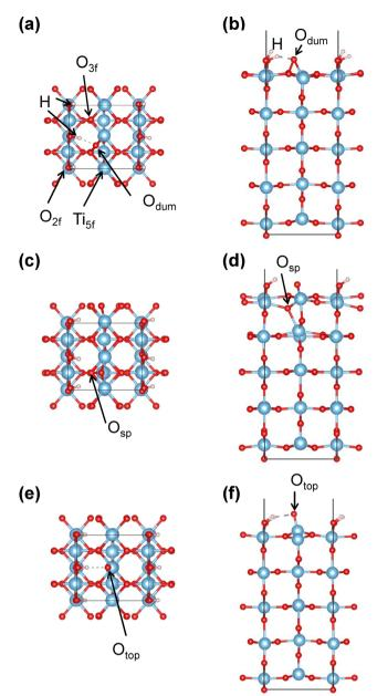
Fig. 4 Geometry of metastable adsorbed O configurations with coadsorbed bridging hydroxyls on TiO<sub>2</sub>(110) terraces, including (a) and (b) dumbbell ( $O_{dum}$ ), (c) and (d) split ( $O_{sp}$ ) and (e) and (f) on-top ( $O_{top}$ ). Panels (a), (c) and (e) show top views and (b), (d) and (f) show side views. Shading colors respectively represent blue for Ti, red for O, and white for H.
