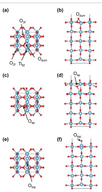
Fig. 3 Geometry of metastable adsorbed O configurations on pristine  $TiO_2(110)$  terraces, including (a) and (b) dumbbell ( $O_{dum}$ ), (c) and (d) split  $(O_{sp})$  and (e) and (f) on-top  $(O_{top})$ . Panels (a), (c) and (e) show top views and (b), (d) and (f) show side views. Shading colors respectively represent blue for Ti and red for O.
