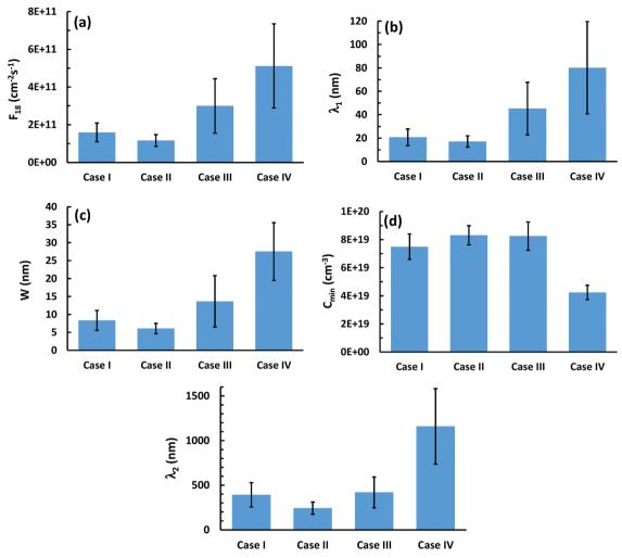
Fig. 2 Bar graphs showing means and standard deviations for profile metrics in each of the four cases: (a)  $F_{18}$  (b)  $\lambda_1$  (c) W (d)  $C_{min}$  (e)  $\lambda_2$ . For all metrics, conditions are 70 °C, t = 60 min.
