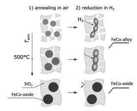
Fig. 7 Schematic representation of the annealing process.
