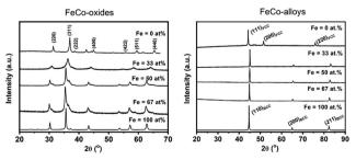
Fig. 1  $\,$  XRPD patterns of the nanostructured FeCo-oxides before (left) and after (right) the reduction process in  $H_2$ .
