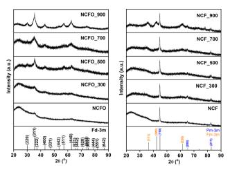
Fig. 3 (Left) XRPD patterns of the samples obtained by the sol-gel selfcombustion synthesis and after thermal treatment at 300 °C, 500 °C, 700 °C, and 900 °C for 1 h in air. (Right) corresponding XRPD patterns after treatment in H2 at 500 °C for 5 h.
