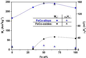
Fig. 2 Saturation magnetization,  $M_{\rm S}$ , and coercivity,  $\mu_0 H_{\rm c}$ , of different samples of nanostructured FeCo-oxides before (black dots) and after (blue dots) the reduction process in  $H_2$  atmosphere.
