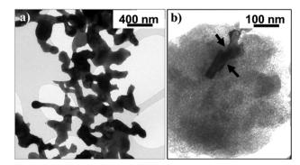
TEM images of the CoFe-alloy with 50 at% (left, (a)) and the CoFealloy/SiO<sub>2</sub> (NCF) composite (right, (b) obtained by the NCFO sample reduction.
