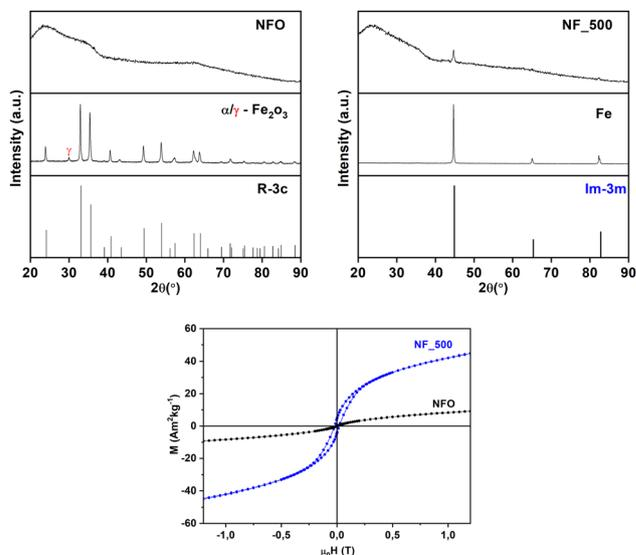
Fig. 8 XRPD patterns of the iron-based samples obtained by the sol-gel self-combustion synthesis (top, left) and after thermal treatment in  $\text{H}_2$  (top, right). Field dependence of magnetization at 300 K for NFO and NF\_500 samples (bottom).
