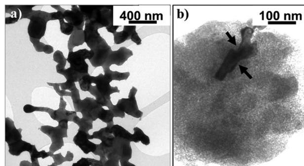
Fig. 4 TEM images of the CoFe-alloy with 50 at% (left, (a)) and the CoFe-alloy/SiO<sub>2</sub> (NCF) composite (right, (b)) obtained by the NCFO sample reduction.
