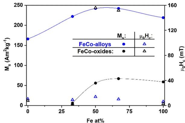
Fig. 2 Saturation magnetization,  $M_s$ , and coercivity,  $\mu_0 H_c$ , of different samples of nanostructured FeCo-oxides before (black dots) and after (blue dots) the reduction process in  $H_2$  atmosphere.
