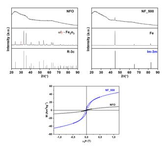
Fig. 8 XRPD patterns of the iron-based samples obtained by the sol-gel self-combustion synthesis (top, left) and after thermal treatment in  $H_2$  (top, right). Field dependence of magnetization at 300 K for NFO and NF\_500 samples (bottom).
