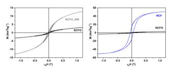
**Fig. 6** Magnetization (*M*) vs. applied field (*H*) at 300 K for NCFO/NCFO\_900 (left), and NCF/NCFO (right).
