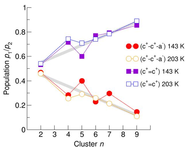
**Fig. 4** Populations  $q_1$  of ( $c^+-a^-$ ) H-bonds and  $q_2$  of ( $c^+=c^+$ ) H-bonds in carboxy-functionalized ionic liquids [DOOC-(CH<sub>2</sub>)<sub>n</sub>-py][NTf<sub>2</sub>] with  $n = 2, 4, 5, 6, 7,$  and  $9$ , derived from NMR solid-state spectra at 143 K (open symbols) and 203 K (closed symbols). At  $n = 9$ , the population is almost solely governed by ( $c^+=c^+$ ) H-bonds.
