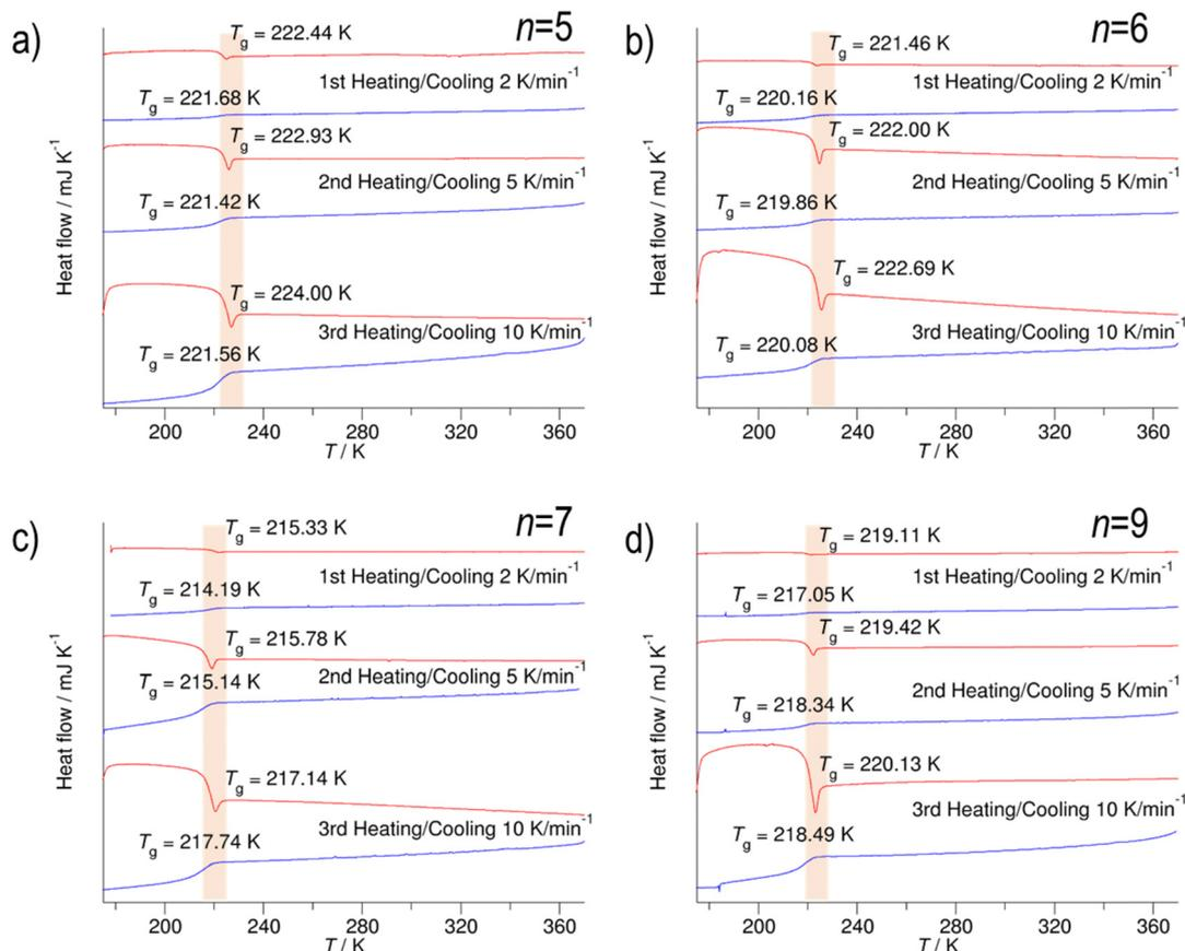
Fig. 1 The DSC thermograms of the ILs [HOOC-(CH<sub>2</sub>)<sub>n</sub>-py][NTf<sub>2</sub>] with (a)  $n = 5$ , (b)  $n = 6$ , (c)  $n = 7$  and (d)  $n = 9$ , showing supercooling and finally glass transitions, indicated by the glass transition temperatures,  $T_g$ , between 215 and 220 K.
