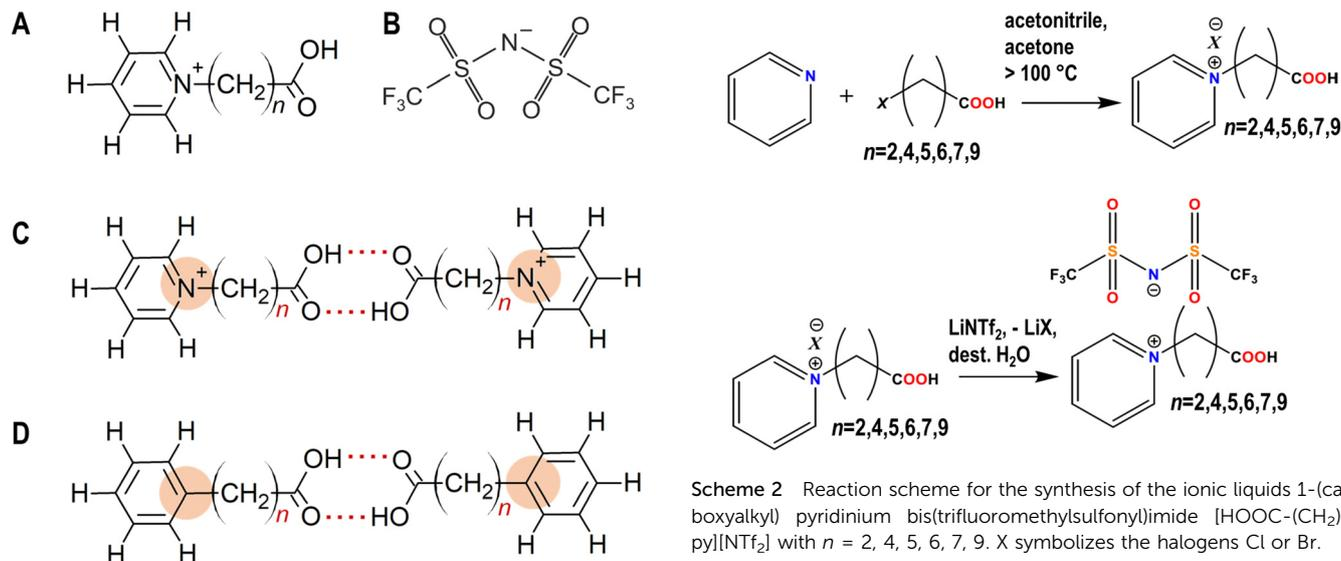
**Scheme 2** Reaction scheme for the synthesis of the ionic liquids 1-(carboxyalkyl)pyridinium bis(trifluoromethylsulfonyl)imide [HOOC-(CH<sub>2</sub>)<sub>n</sub>-py][NTf<sub>2</sub>] with *n* = 2, 4, 5, 6, 7, 9. X symbolizes the halogens Cl or Br.
