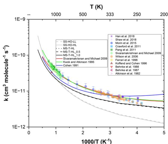
Fig. 6 Rate constants of the overall reaction  $n$ -heptane + OH as a function of temperature. Black and grey lines are our calculated rate constants, other lines are from estimations, while the symbols represent experimental data from the literature with their associated uncertainties when available.
