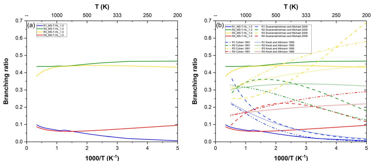
Fig. 7 Branching ratios of the *n*-heptane + OH reaction: (a) our MS-T-HL\_1.0 results in solid lines only and (b) compared to estimations in interrupted lines.<sup>14,17,18</sup>
