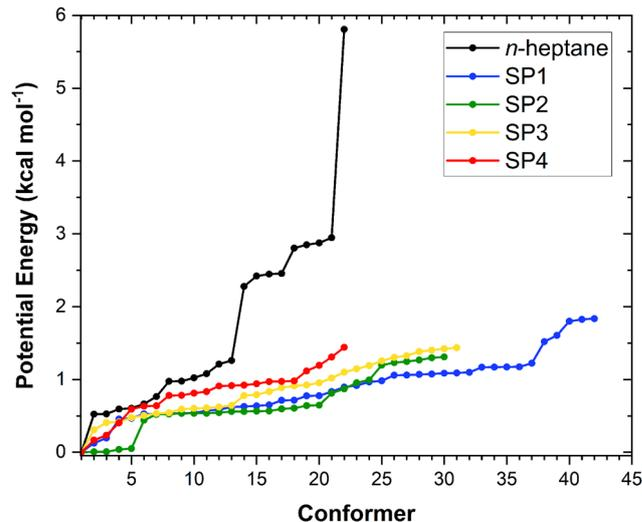
Fig. 2 Potential energy distribution of the conformers of the *n*-heptane and saddle point (SP) species of reactions (R1)–(R4) at the M06-2X/aug-cc-pVTZ level. Energy values are defined with respect to that of the lowest-energy conformer of the corresponding stationary point.
