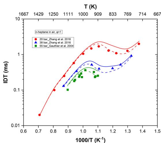
Fig. 8 Comparison of *n*-heptane ignition delay time predictions at  $\phi = 1$ ,  $p = 20$  bar,  $p = 38$  bar, and  $p = 55$  bar. Symbols are experiments<sup>2,41</sup> while solid and dashed lines respectively correspond to simulations with and without the implementation of the updated rate constants for reactions (R1)–(R4) in the original mechanism.<sup>2</sup>
