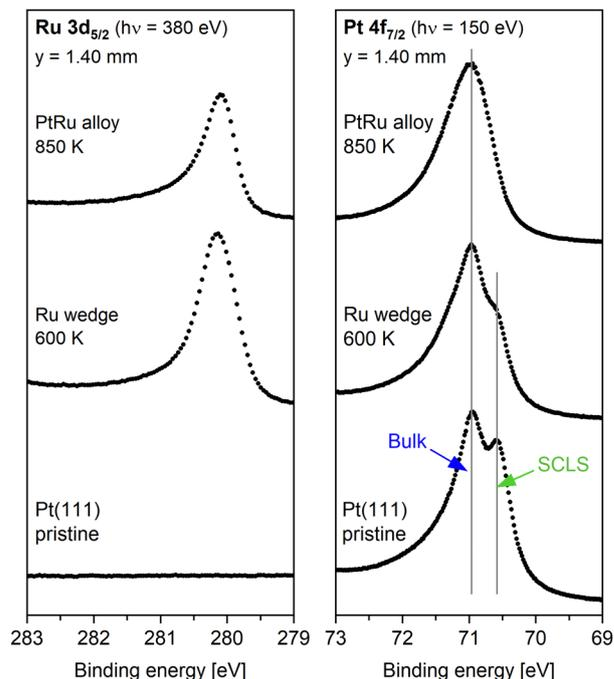
Fig. 1 Comparison of the observed Ru 3d<sub>5/2</sub> and Pt 4f<sub>7/2</sub> spectra at different stages of the experiment, recorded at the position *y* = 1.40 mm. From bottom to top: pristine Pt(111) substrate; after deposition of the Ru wedge and flash-annealing to 600 K; after subsequent flash-annealing to 850 K.
