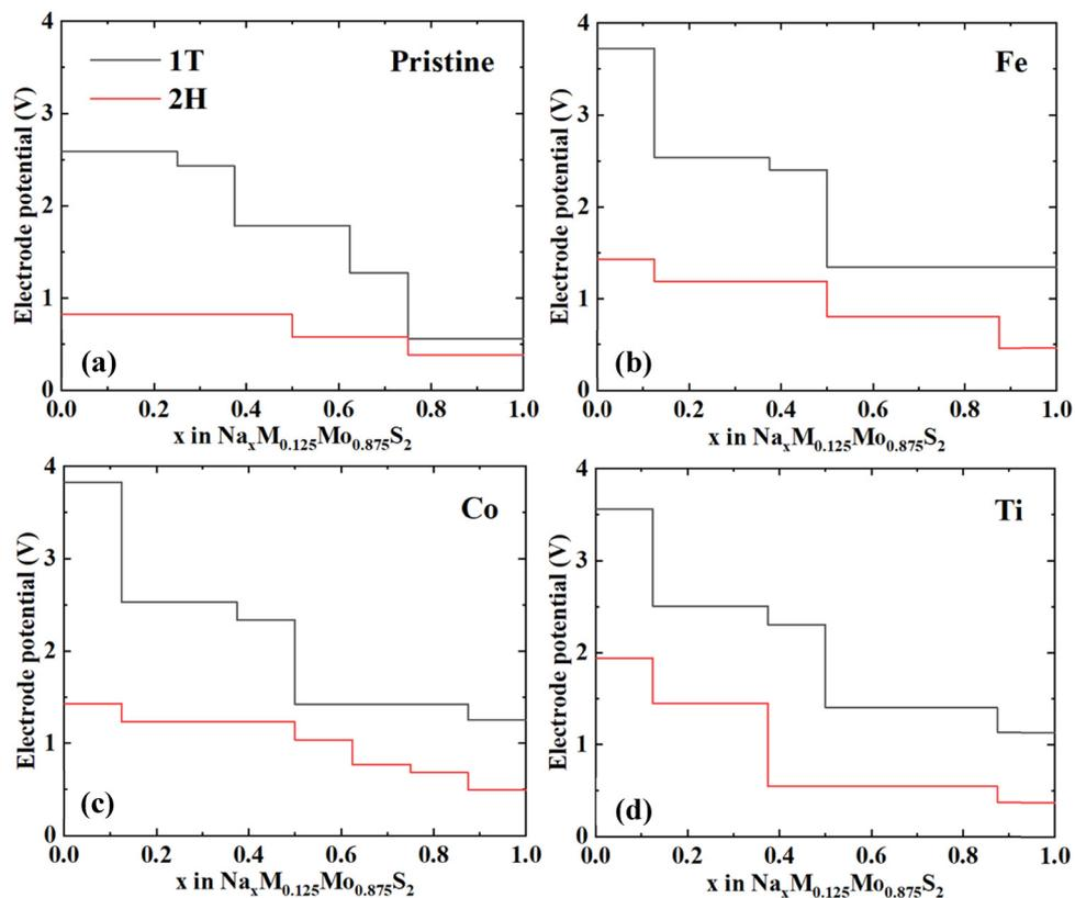
Fig. 7 OCV curves of 1T and 2H phase (a) pristine, (b) Fe, (c) Co, and (d) Ti doping  $\text{MoS}_2$  structures.
