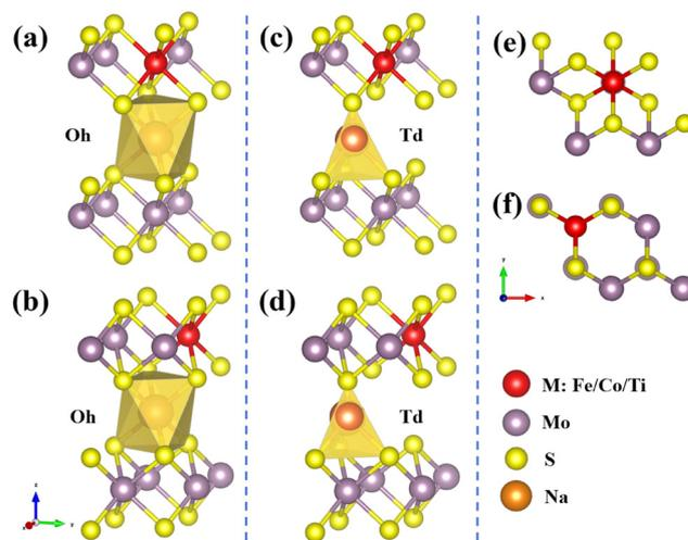
Fig. 1 Octahedral binding sites of Na in the (a) 1T and (b) 2H phase MoS<sub>2</sub>, tetrahedral binding sites of Na in the (c) 1T and (d) 2H phase MoS<sub>2</sub>, and the top view of TM-doped multi-layered (e) 1T and (f) 2H phase MoS<sub>2</sub>.
