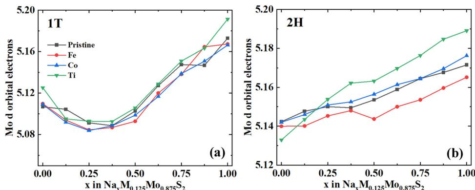
Fig. 5 Mo d orbital electrons of (a) 1T and (b) 2H phase pristine MoS<sub>2</sub> and  $\text{M}_{0.125}\text{Mo}_{0.875}\text{S}_2$ , M: Fe/Co/Ti.
