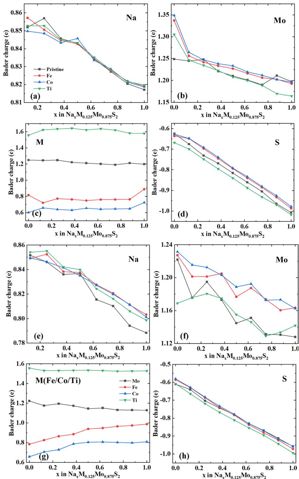
Fig. 4 Bader charge for (a) Na, (b) Mo, (c) M and (d) S in the 1T phase, and (e) Na, (f) Mo, (g) M and (h) S in the 2H phase of pristine  $\text{MoS}_2$  and  $\text{Na}_{0.125}\text{Mo}_{0.875}\text{S}_2$ , M: Fe/Co/Ti and the black lines in (c) and (g) are the average charge of Mo in pristine  $\text{MoS}_2$ .
