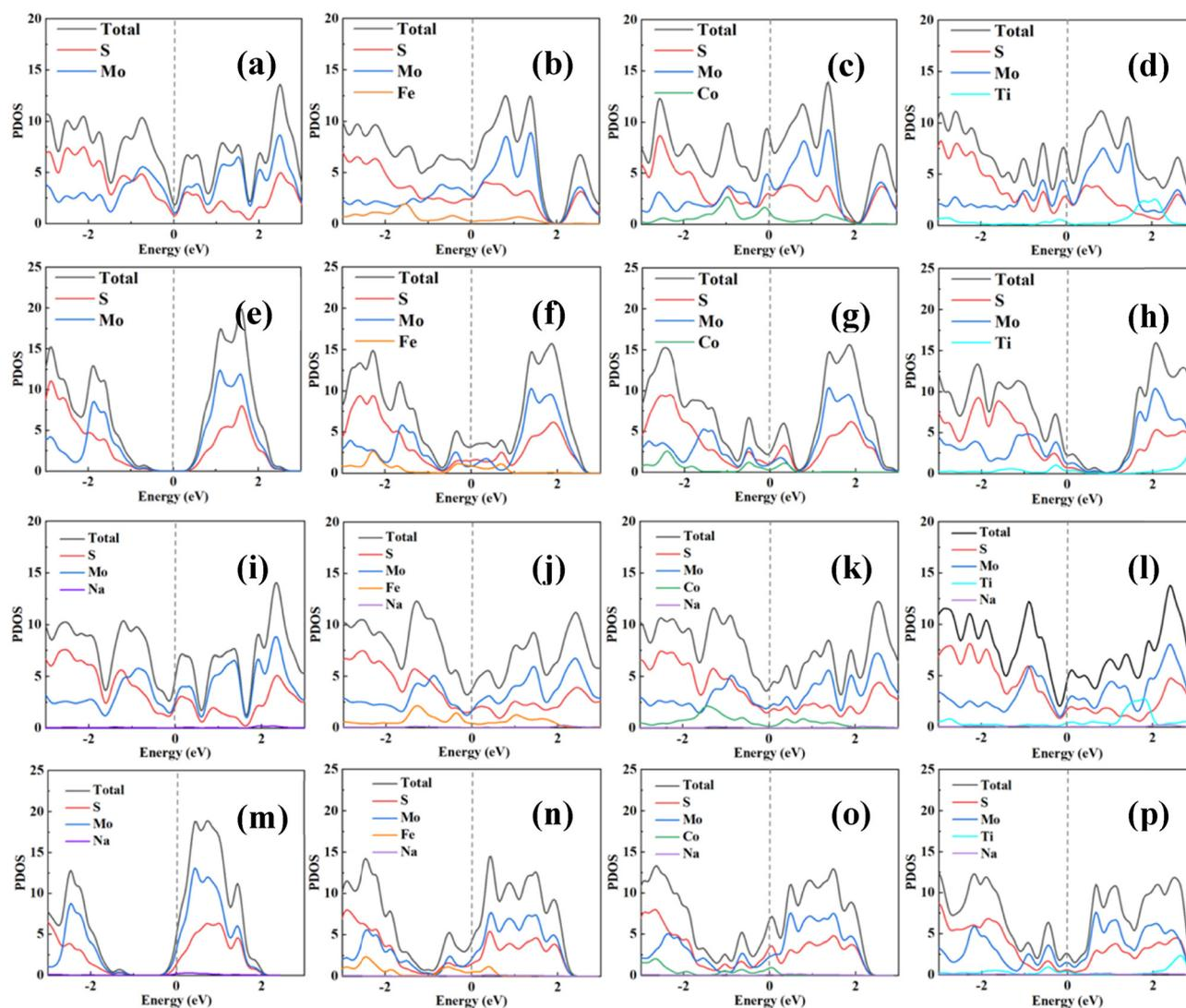
Fig. 8 Projected density of states for (a) pristine, (b) Fe-doped, (c) Co-doped and (d) Ti-doped 1T phase  $\text{MoS}_2$  and (e) pristine, (f) Fe-doped, (g) Co-doped and (h) Ti-doped 2H phase  $\text{MoS}_2$ . Na atom intercalation in (i) pristine, (j) Fe-doped, (k) Co-doped and (l) Ti-doped 1T phase  $\text{MoS}_2$  and Na atom intercalation in (m) pristine, (n) Fe-doped, (o) Co-doped, and (p) Ti-doped 2H phase  $\text{MoS}_2$ . The Fermi level is set to zero eV.
