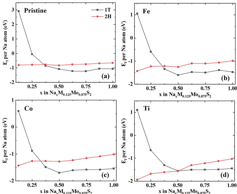
Fig. 3 Formation energy per Na atom for 1T and 2H phases of (a) pristine, (b)  $\text{Fe}_{0.125}\text{Mo}_{0.875}\text{S}_2$ , (c)  $\text{Co}_{0.125}\text{Mo}_{0.875}\text{S}_2$ , and (d)  $\text{Ti}_{0.125}\text{Mo}_{0.875}\text{S}_2$ .
