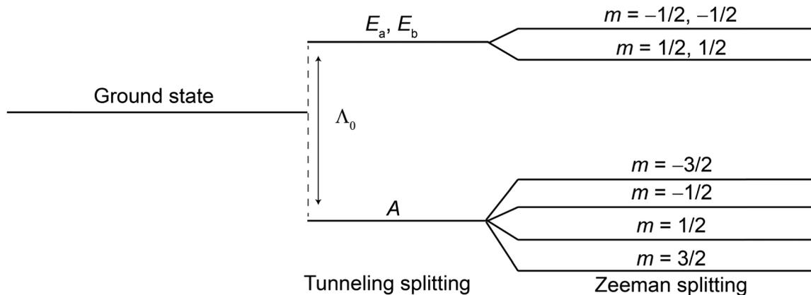
**Scheme 1** Spin-states ground state energy level scheme for an isolated  $\text{CF}_3$  group (without including the coupling to the  $^{13}\text{C}$  spin, adapted from ref. 38). The energy difference between the  $A$  and  $E_a, E_b$  manifolds is the tunneling splitting  $\Lambda_0$ .
