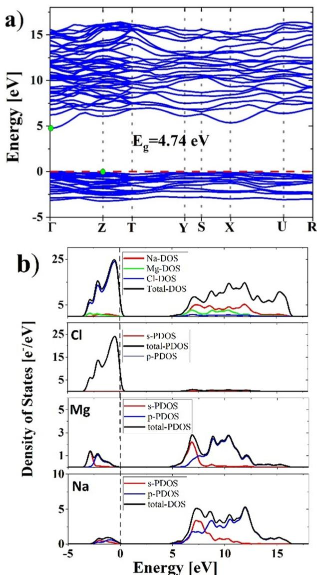
Fig. 2 (a) Band structure and (b) density of states of the  $\text{Na}_2\text{MgCl}_4$  structure; dashed red and black lines represent the Fermi level. Green bullets in (a) represent the valence band maximum at the Z point and conduction band minimum at the  $\Gamma$  point.
