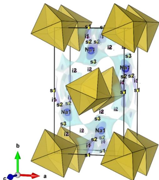
Fig. 4 3D network of  $\text{Na}^+$  migration pathways in  $\text{Na}_2\text{MgCl}_4$  (blue iso-surfaces) calculated using BVSE computations. Yellow polyhedra represent the  $[\text{MgCl}_6]$  octahedra.
