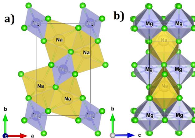
Fig. 1 Unit cell of  $\text{Na}_2\text{MgCl}_4$  in the conventional representation (space group Pbam, No. 55): (a) and (b) views along the [001] and  $[\bar{1}00]$  directions, respectively. Blue and green spheres represent the  $\text{Mg}^{2+}$  and  $\text{Cl}^-$  ions, while blue and orange polyhedra represent the  $[\text{MgCl}_6]$  and  $[\text{NaCl}_6]$  octahedra, respectively.
