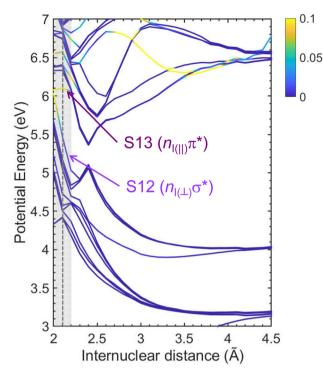
Fig. 7 Computed XMS-CASPT2 potential energy curves for vinyl iodide as a function of the C-I distance. The vertical color map indicates the values of the oscillator strength: dark blue indicates the lowest absorption probability while yellow represents the highest absorption probability. The grey box illustrate the Franck-Condon region around the equilibrium geometry indicated by a grey dashed line.
